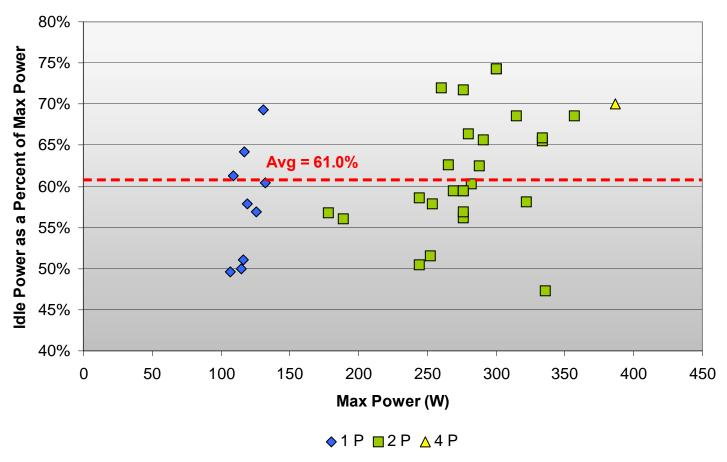
Scaling Idle to maximum power appears to work across processor #s and different power ranges
