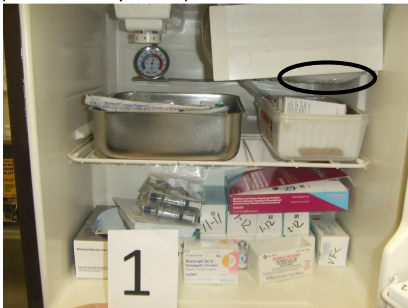
Photo 3: Dorm-Style Unit Used for Permanent VFC Vaccine Storage (Note Frost Buildup in Circle)
