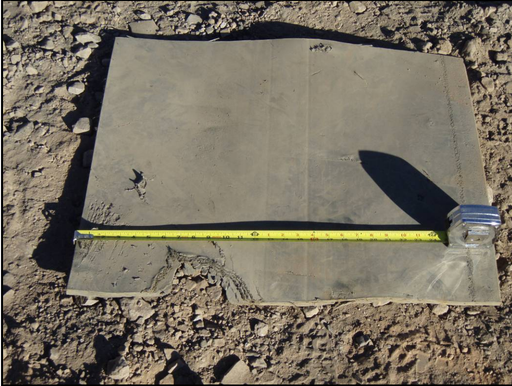
Photo 15 – A 24-inch by 28-inch conveyor belt piece used to patch the 24-inch-diameter aggregate pipe.
