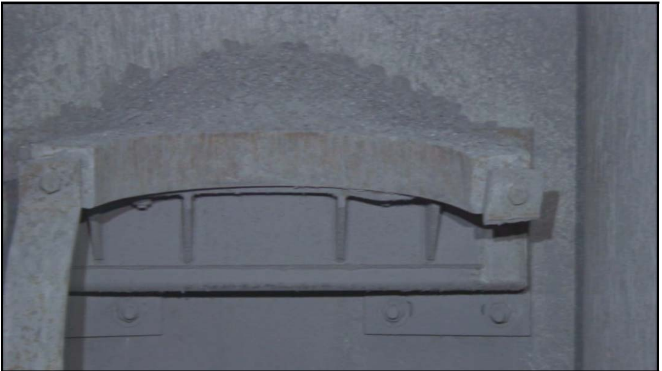
Photo 22 – Video Time 1:09:56 - Clamp sheared at a new bracket location.
