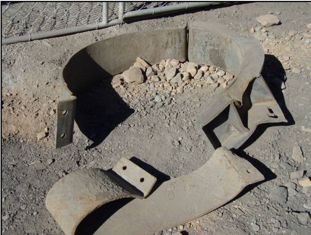
Photo 32 – Two bearing clamps at evidence yard, one of which still attached to clamp bracket.
