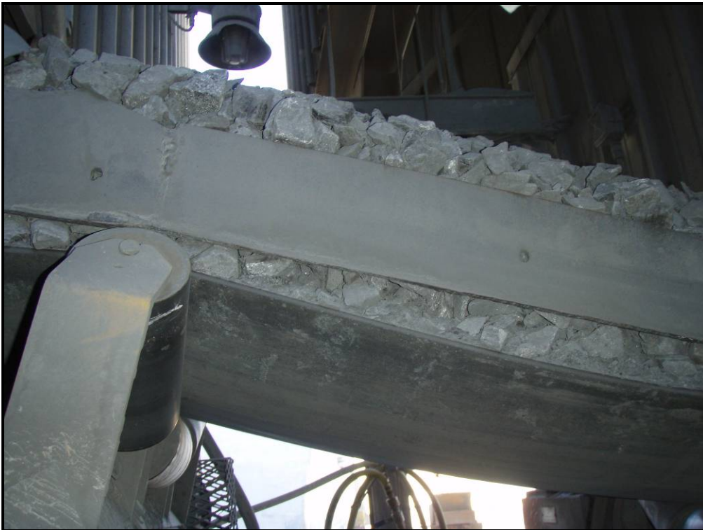
Photo 16 – The 28-inch-wide surface feed conveyor belt overflowing with aggregate.
