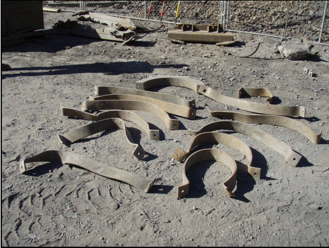
Photo 31 – Single clamps at evidence yard, one of which still attached to a clamp bracket.
