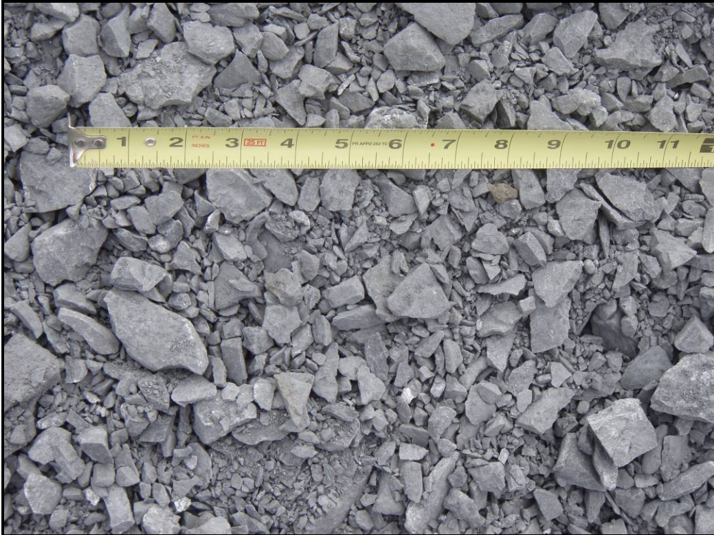
Photo 1 – Minus 3-inch aggregate and fines at surface stockpile near top of ventilation shaft.
