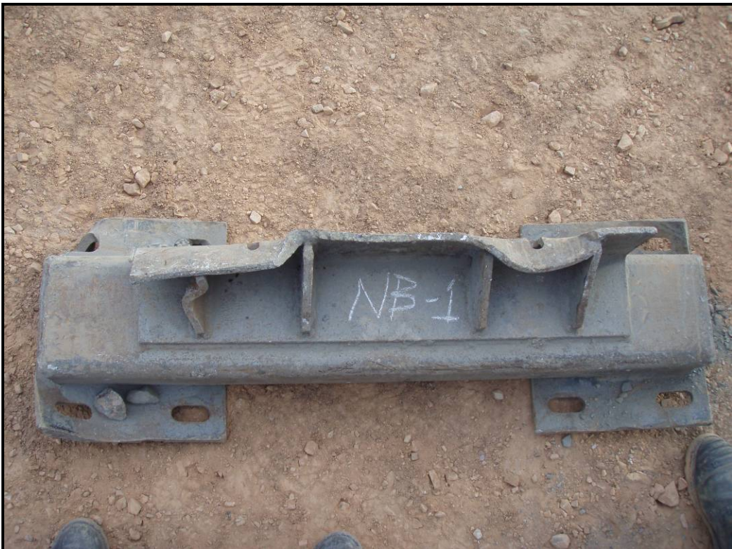
Photo 30 – New bracket (NB-1) at evidence yard. Stiffened angle bent down and stiffener buckled.
