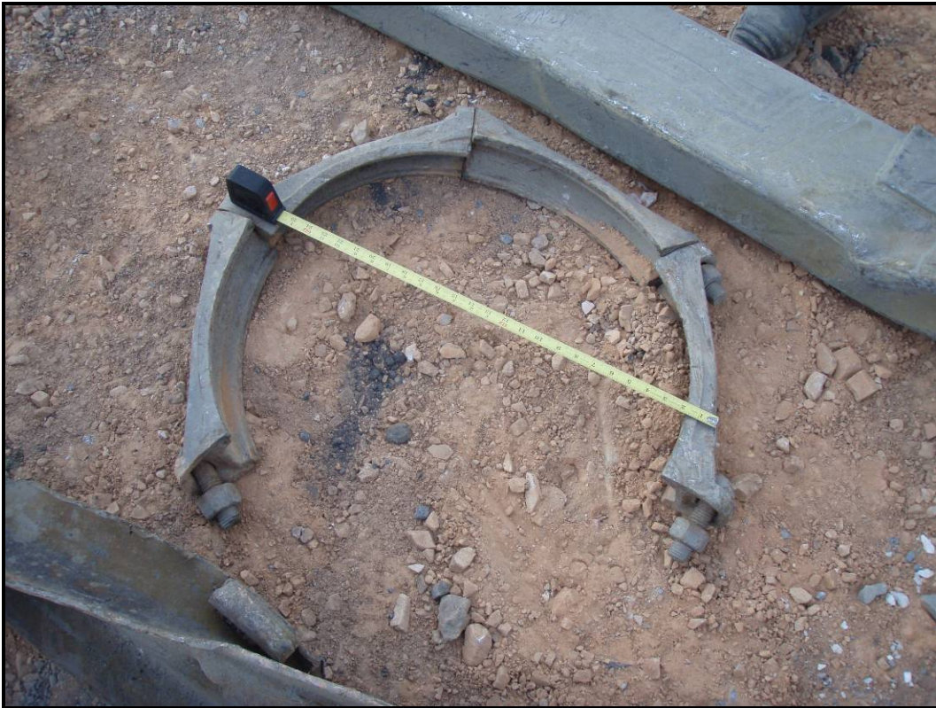
Photo 6 – Partial Victaulic Style 31 coupling for 24-inch-diameter aggregate pipe.
