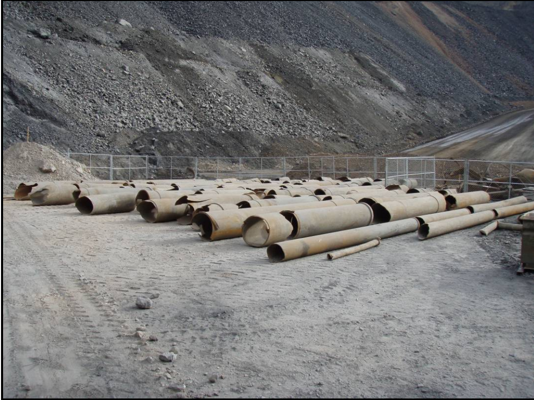
Photo 35 – Recovered 24-inch-diameter partial pipe spools at evidence yard.
