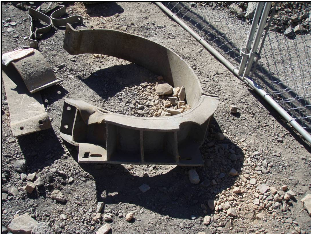
Photo 34 – Bearing clamp bracket and clamp at evidence yard. Additional slot burned in clamp bracket to accommodate misalignment.
