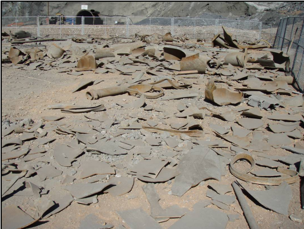
Photo 36 – Pipe shards from 24-inch-diameter aggregate pipe at evidence yard
