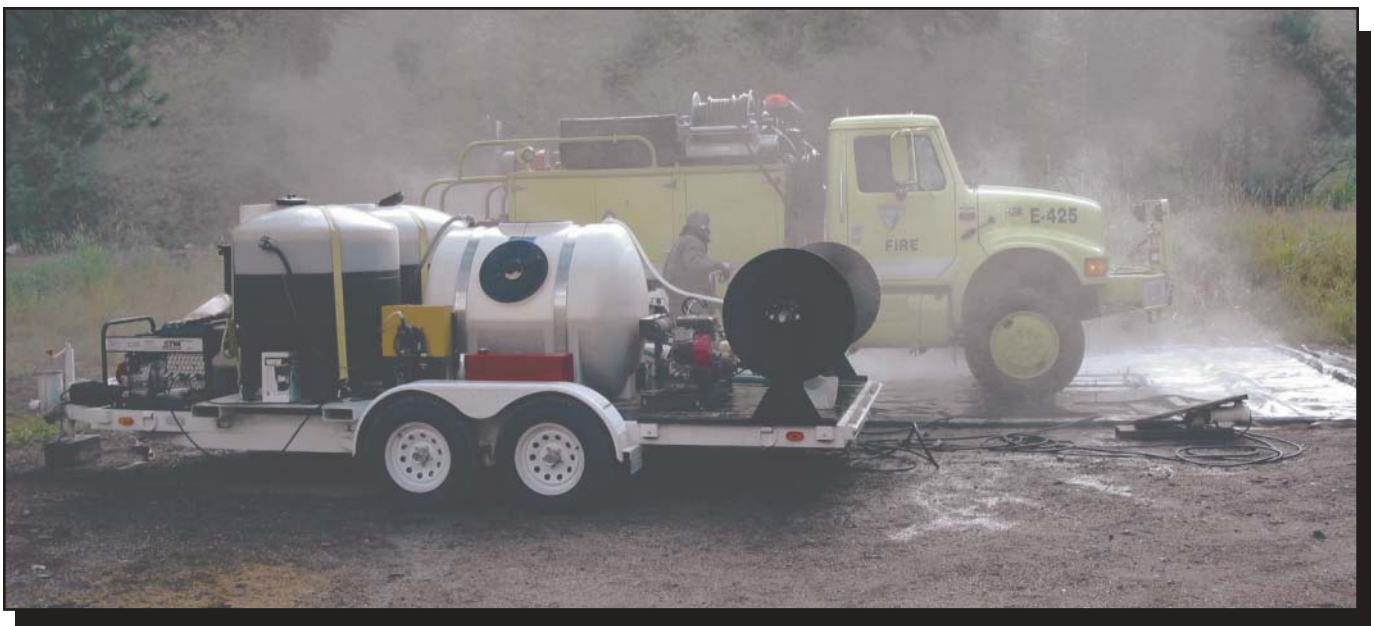
Figure 9—The portable vehicle washer developed by the Missoula Technology and Development Center is being used to clean a fire engine on the Bitterroot National Forest.
