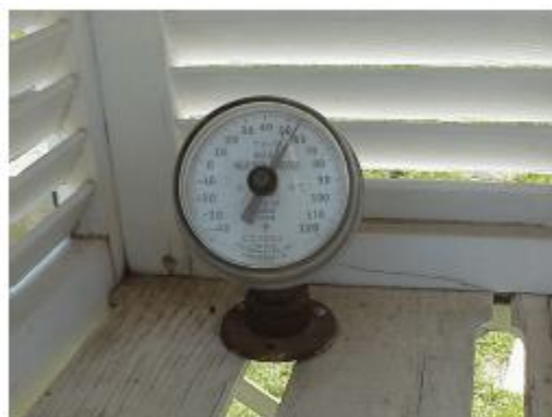
Figure E-2. Palmer Soil Thermometer in Shelter
