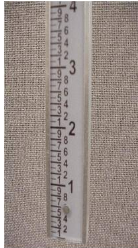
Figure A-53. Snow Stick Graduated Scale to One Tenth of an Inch
