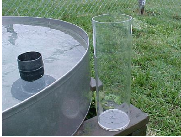
Figure D-4. Transparent Measuring Tube and Stilling Well Inside the Pan
