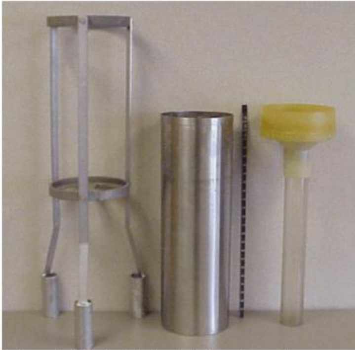
Figure A-4. Eight-Inch Precipitation Gauge Components
