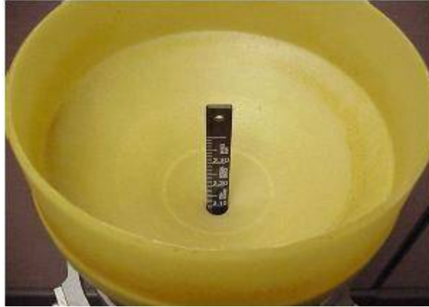
Figure A-50. Eight-Inch Gauge with Measuring Stick Inserted
