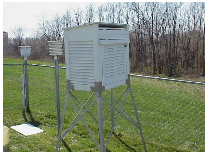
Figure B-2 - Instrument Shelters Cotton Region Shelter and Two MMTS Shelters
