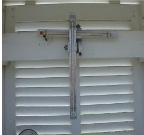
Figure B-9 - Maximum Thermometer in Reading Position
