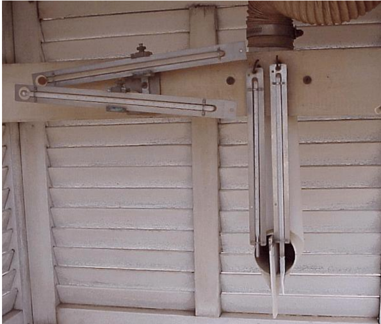
Figure D-9. Dry and Wet-bulb Thermometers in CRS
