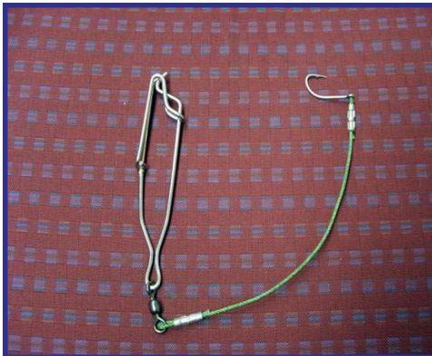
-USFWS The Columbia Fishery Resources Office has adapted the use of ganion clips with swivels for use with set lines. The pre-baited hook units are attached to the main line as it is deployed, minimizing tangles and providing a safer work environment.
