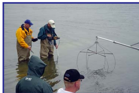
-GLFC by Michael Fodale Instructors Jim Reynolds (upper left) and Jim Boardman (upper right) conduct measurements of the electrical parameters from a boomshocking boat during National Conservation Training Center sponsored Principles and Techniques of Electrofishing course.
