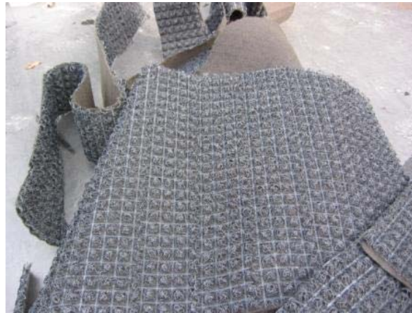
FIGURE 7: Example of fabric drainage mat. 13
