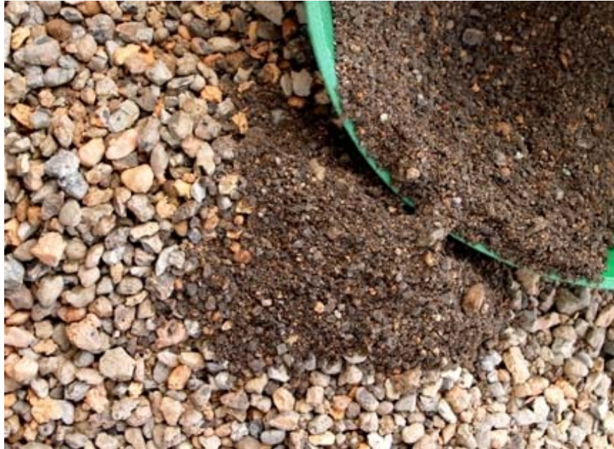
FIGURE 10: Example of light-weight growing medium (expanded slate, bark and compost). 16
