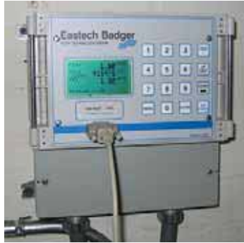
Figure 3.4. Eastech Badger 4400 Flow Meter/Data Logger
