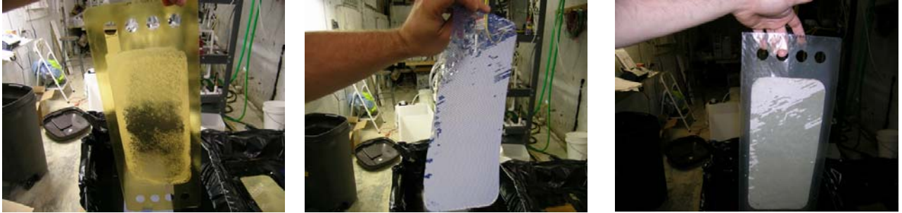
Figure 6. Photographs from left to right of the CMX membrane above the \text{CaCl}_2 compartment, the spacer in the \text{CaCl}_2 compartment, and the ACS membrane below the \text{CaCl}_2 compartment
