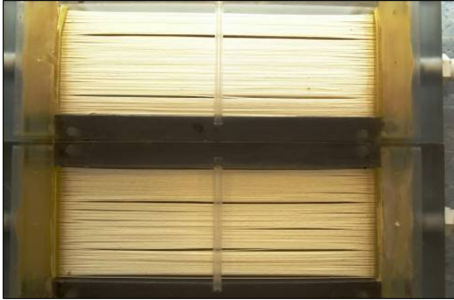
Figure 16. Photo of fiber bunching leading to fluid channeling on the DCMD module shell side.
