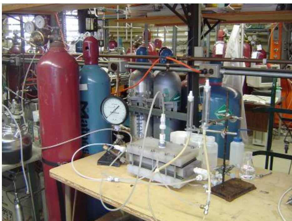
Figure 6b. Photograph of the membrane gas permeation measurement experimental setup of figure 6a.
