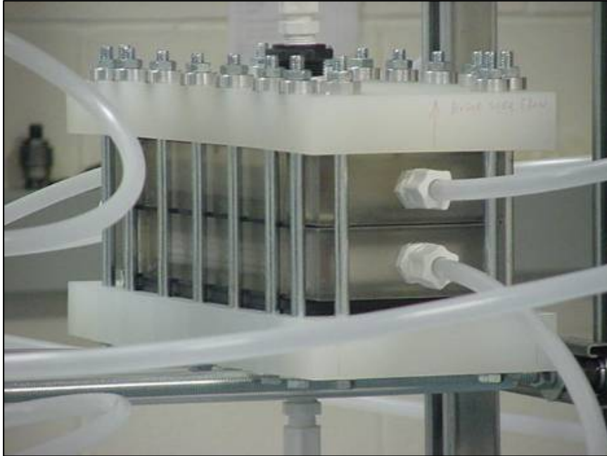
Figure 14. Photo of connections of DCMD modules.
