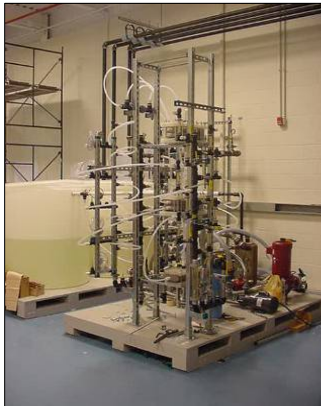
Figure 12b. Photograph of the DCMD pilot-scale demo setup (view from a distance).
