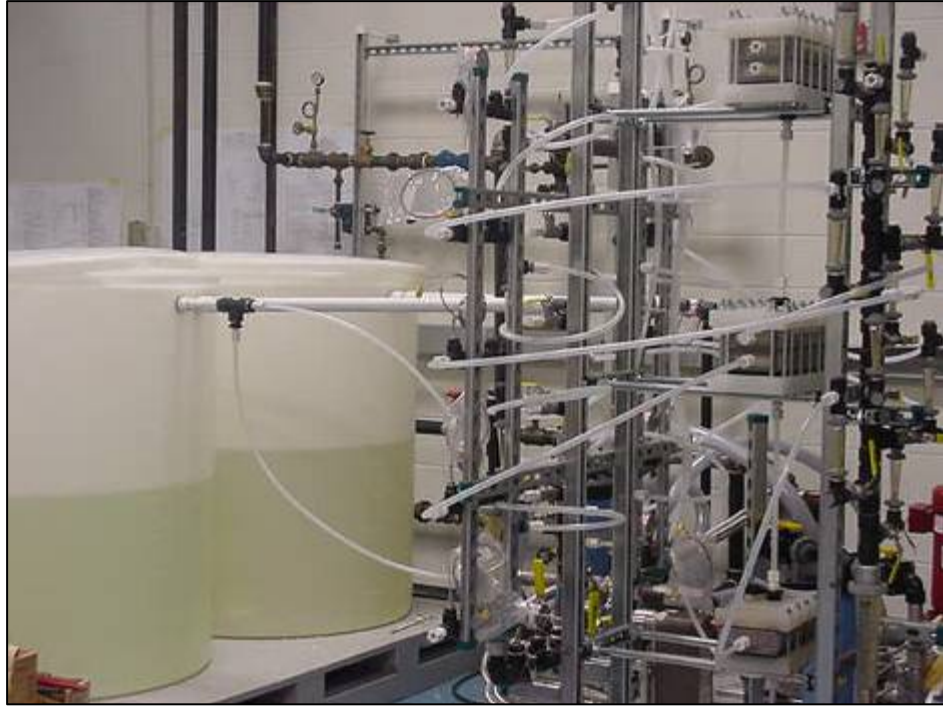
Figure 12a. Photograph of the DCMD pilot-scale demo setup.
