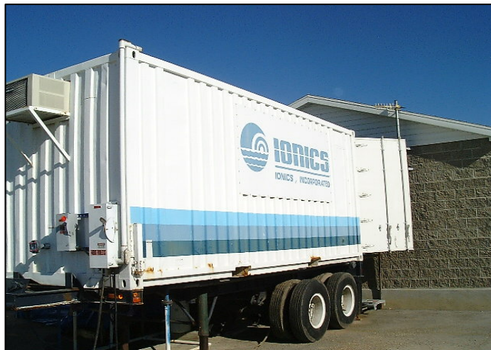
Figure 3-7. EDR pilot unit trailer.
