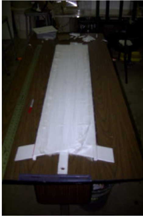
Figure 27.—Basic Heat Transfer Wall of a NEWT Tower Design.
