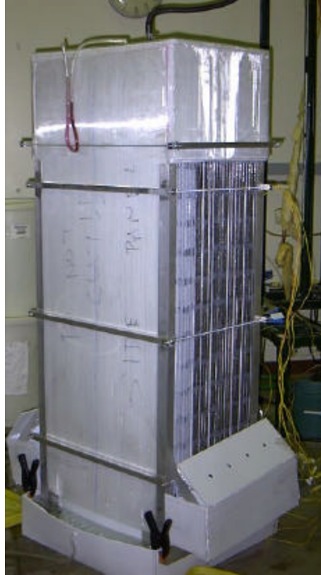
Figure 29.—700 ft 2 NEWT tower Final Sub-Module Produces 125 GPD at f=10 (Note: Eight of these Sub-Modules Comprises 1,000 GPD Demonstration Pilot Plant)
