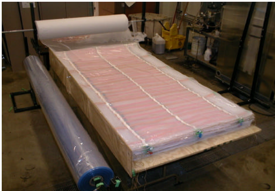
Figure 14.—Completion of the Heat Transfer Envelopes of the Pre-Pilot Unit.
