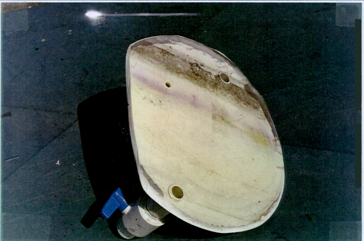
Figure 6-5: Detail of Crystallizer End Cap Rupture
