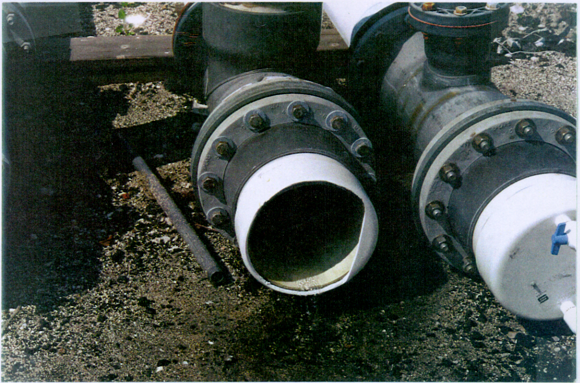
Figure 6-5: Detail of Crystallizer End Cap Rupture
