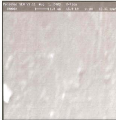
Fig. 12: element 02A217 – inner surface of defective membrane in segment 7 10.000 x
