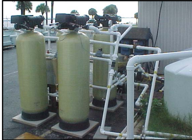
Figure 3-3. Multimedia Filtration Pilot Unit – East Coast Site.
