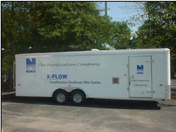
Photo 3 – Ultrafiltration Pretreatment Pilot Trailer.
