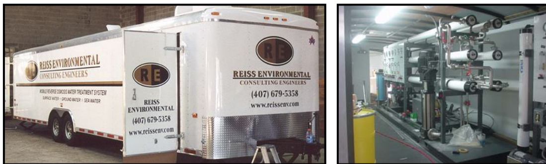
Figure 3-6. Reiss Environmental Trailer-Mounted SWRO Pilot Plant.
