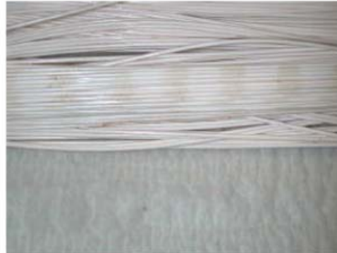
Fig. 9: element 02A217 – membrane bundle
