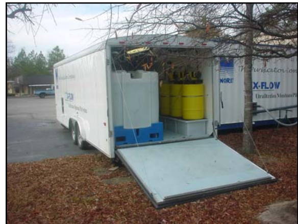
Photo 4 – Ultrafiltration Pilot (rear view)
