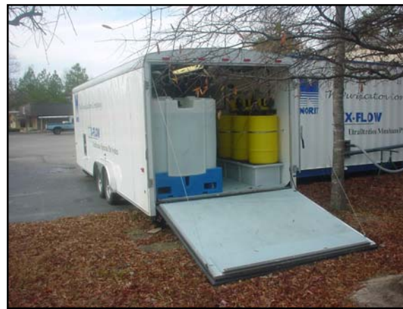
Photo 4 – Ultrafiltration Pilot (rear view).
