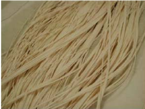
Fig. 8: element 02A217 – membrane bundle
