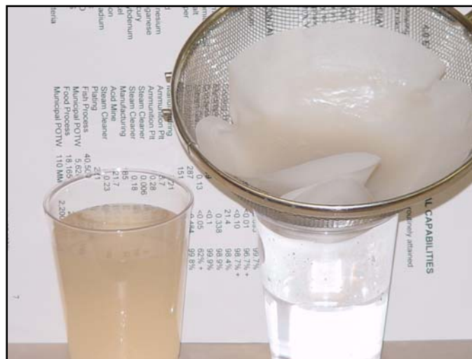
Figure 7.3 Tannic/humic acid feed solution (on left) and treated, filtered solution (on right).
