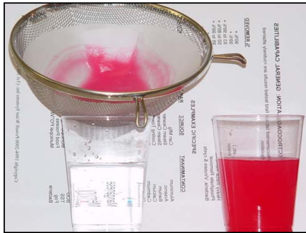
Figure 7.2 Treated filtered solution (on left) and EC feed solution (on right) for latex paint test run.
