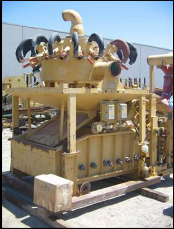
Desanding and desilting equipment (photo by GEOSCIENCE).
