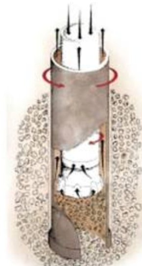
Dual rotary drilling method with dual-tube inner drill string (Foremost Industries, LP, 2003).
