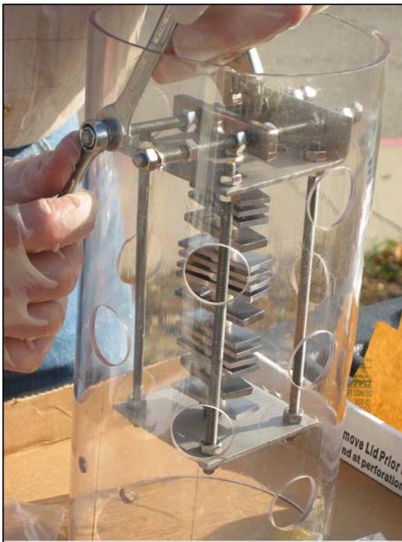
Downhole metal coupon rack used for corrosion testing (photo by GEOSCIENCE).
