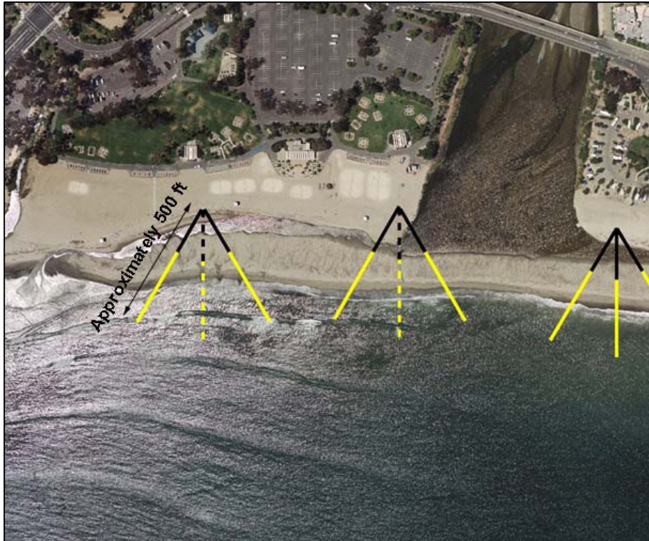
Three slant well clusters with three slant wells per cluster. Dashed lines indicate backup wells (GEOSCIENCE, 2007).
