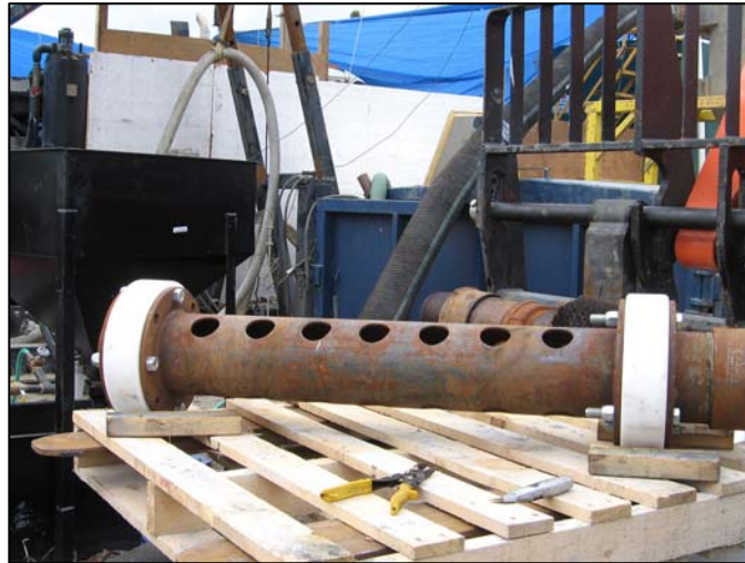
Swabbing tool with UHMW packers (photo by GEOSCIENCE).
