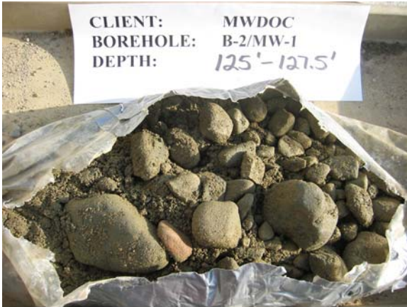
Sonic core samples showing coarse-grained formation materials (photos by GEOSCIENCE).
