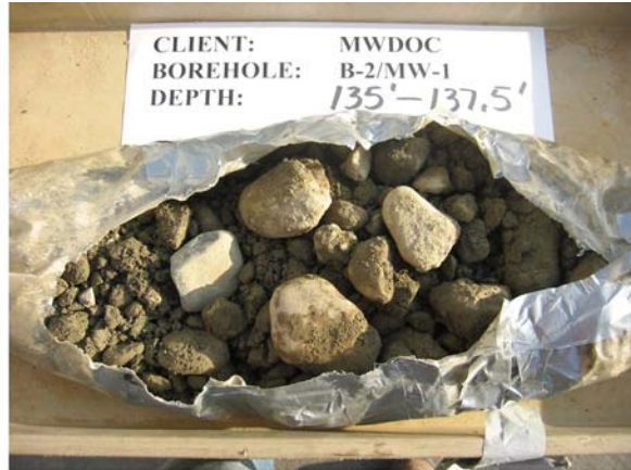
Sonic core samples showing coarse-grained formation materials (photos by GEOSCIENCE).
