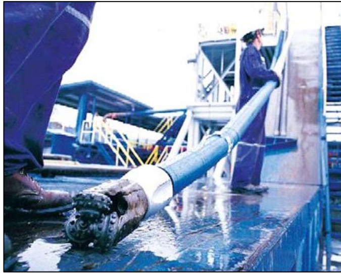
Portion of bottom hole assembly (drill bit, bent subassembly and mud motor) (Hill et al., 1996).
