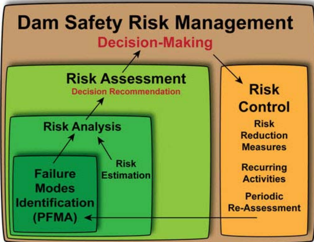
Figure 1. Dam Safety Risk Management Components
