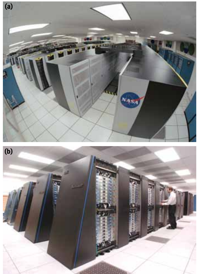
Fig. 1: Two highly parallel machines that have been used in the NIST simulation program: (a) Columbia, a cluster of 24 SGI Altix machines, each containing 512 processors, maintained by the National Aeronautics and Space Administration (NASA); and (b) Intrepid, an IBM Blue Gene/P with 163,840 processors, maintained by Argonne National Laboratory. Time on these machines was awarded to us by the NASA National Leadership Computing System initiative and by the DOE Innovative and Novel Computational Impact on Theory and Experiment (INCITE) program, respectively. The machines are identified only to adequately describe the project—the identification is not an endorsement or recommendation by NIST, nor does it mean that the equipment is necessarily the best available for the purpose
