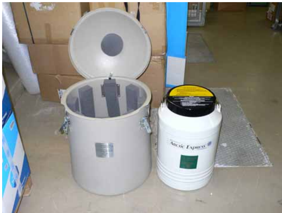
Fig A11.1. A dry shipper and the protective bin in which it is shipped
