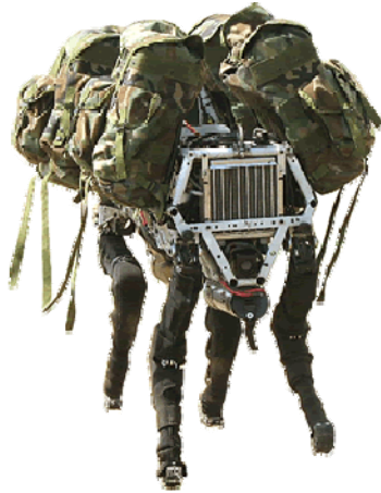
CENTAUR Components: Big Dog Quadruped Robot & BEAR Head and Upper Torso
