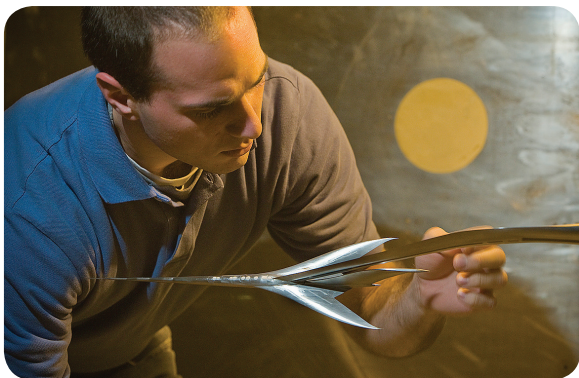
Test engineer Mark D'Aprile checks a small model of a supersonic jet concept designed by Gulfstream Aerospace and tested in a NASA wind tunnel. Image credit: NASA Langley/Sean Smith
