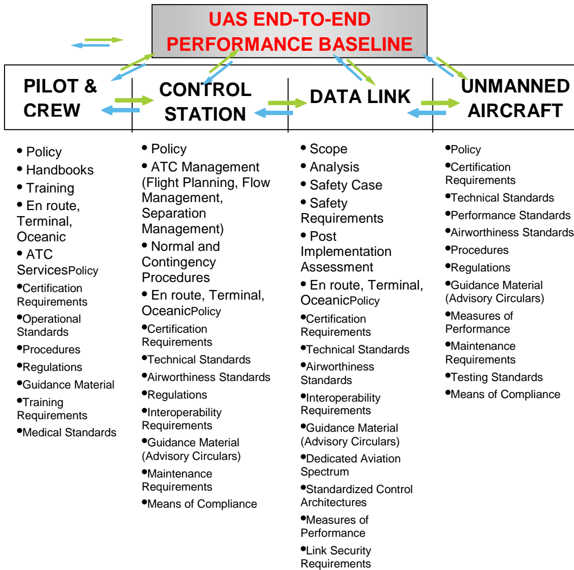
Figure A-1 Product areas relating to UAS that will require supporting research
