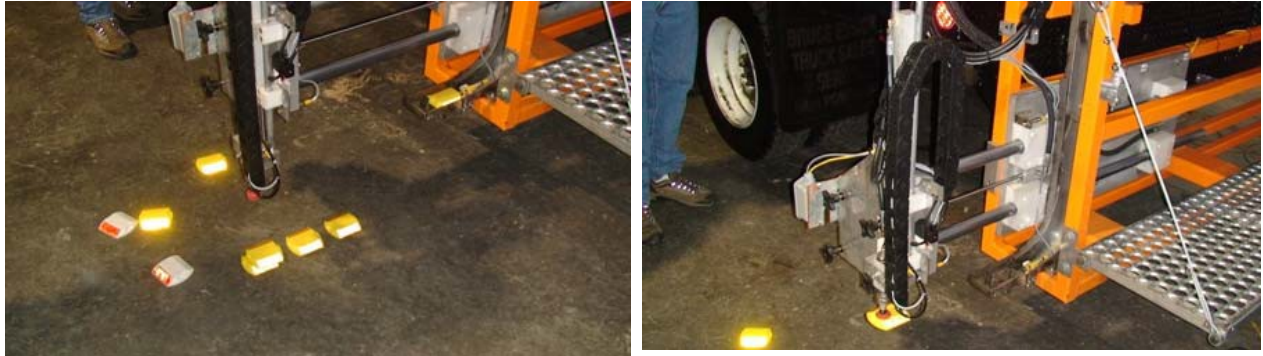
Figure 19. Workshop testing on (a) positioning the marker and (b) picking up and placing the marker.
