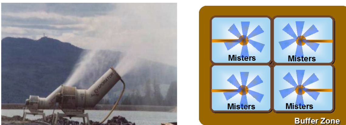
FIGURE 3.3 TYPICAL EVAPORATION POND CONFIGURATION OF MECHANICAL MIST EVAPORATOR
