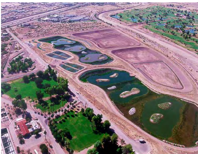
FIGURE 3.16 EXAMPLE OF A SURFACE FLOW CONSTRUCTED WETLAND
