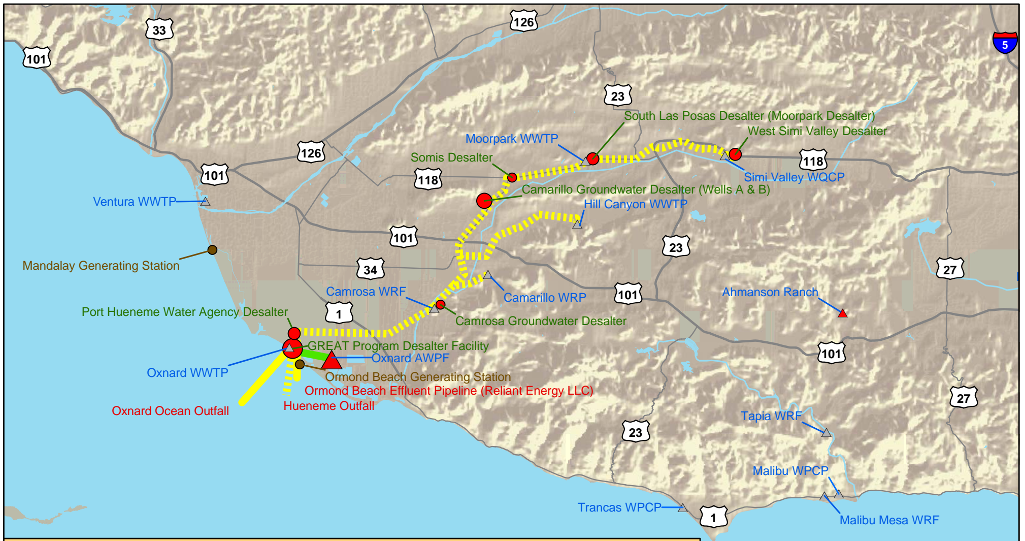
FIGURE 3.4 - WASTEWATER AND GROUNDWATER BRINE-CONCENTRATE SOURCES
