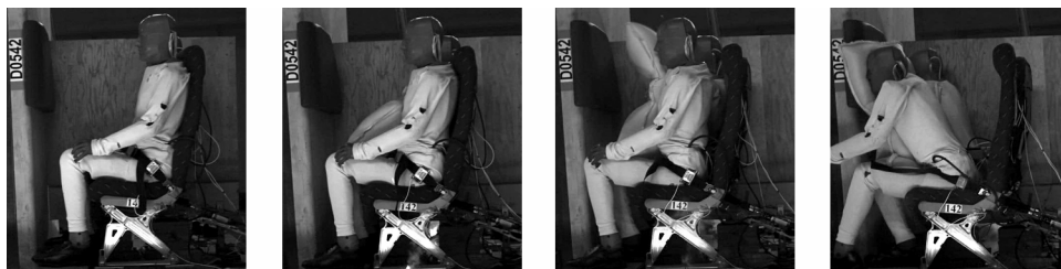
Figure 1: Inflatable Lap Belt Air Bag Inflation Sequence
