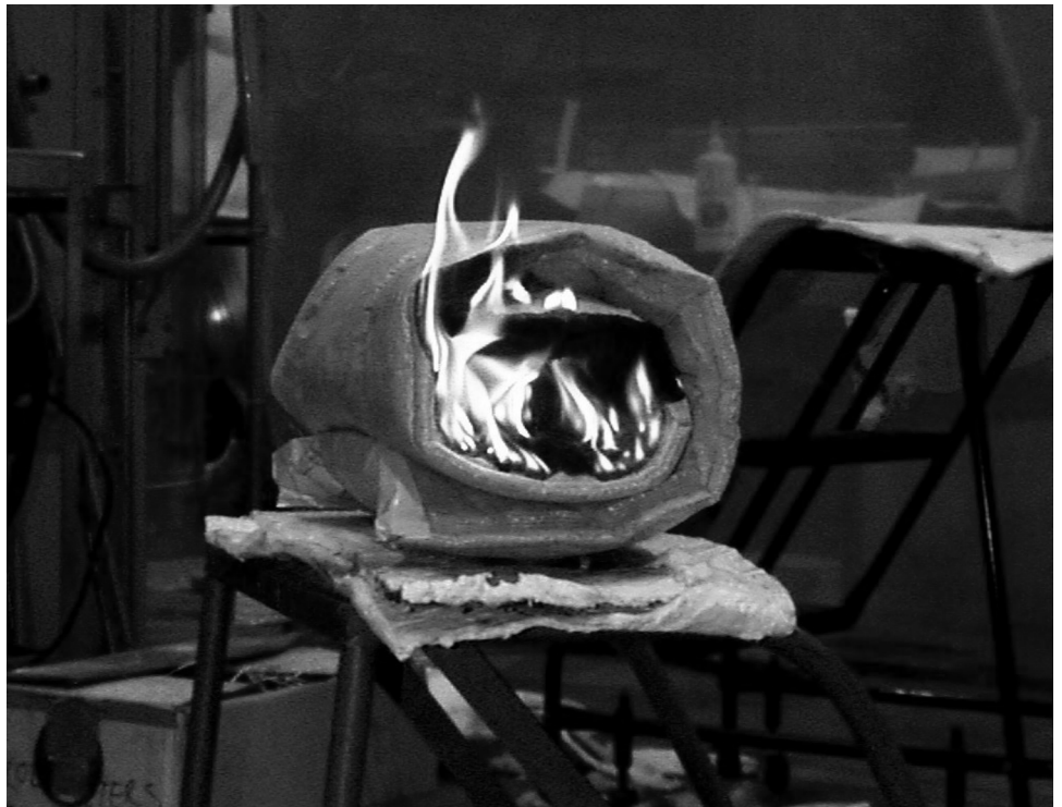
Figure 8: Fire Insulation Blankets
