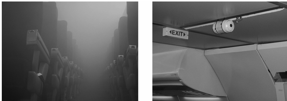
Figure 13: Test Installation of Acoustic Signalling Device
