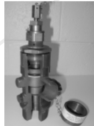
Cut-away of the valve from a halon 1301 total flooding system cylinder. Training aids such as this can be used in technician training courses to provide an understanding of how the systems work. Photo courtesy of U.S. DOD/DLA ODS Reserve.
