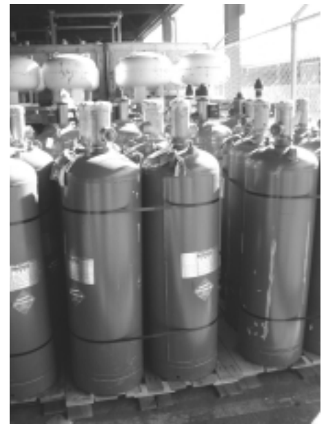
Halon 1301 total flooding system cylinders held in storage. Cylinders such as these are collected from decommissioned systems, and the halon is recycled and banked for critical government and industry programs. Photo courtesy of U.S. Department of Defense (DOD), Defense Logistics Agency (DLA), Ozone Depleting Substance (ODS) Reserve.
