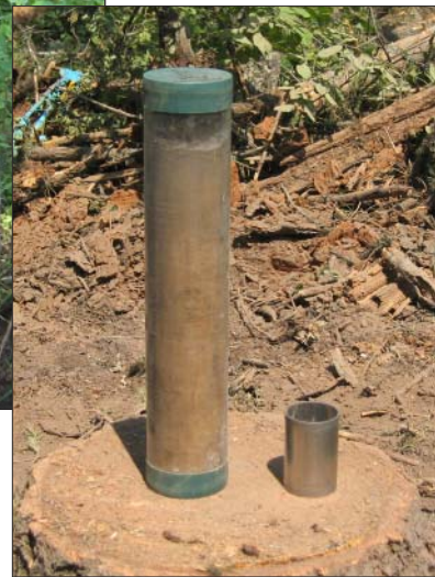
Two types of cores collected with the core sampler. The large core (4 cm x 30 cm) is used to determine pore size distribution at various depths in the mineral soil, and the small core (4 cm x 10 cm) is used to determine bulk density (a measure of compaction). (Photo by Han-Sup Han)
