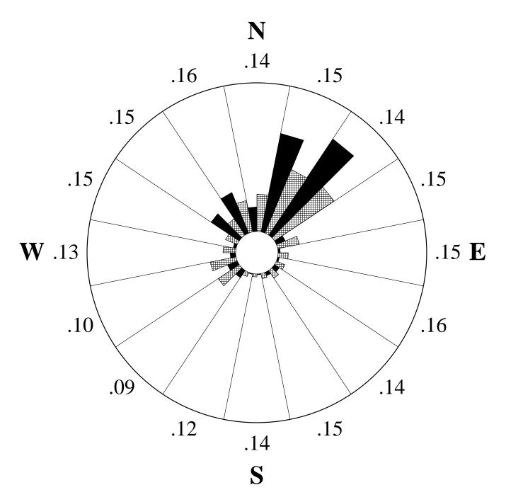
11/5/2001 to 6/30/2005 Wind Rose Ch 1, 7 **SITE 0004** Lone Pine Ridge (New Site) Site Information: Project: New Project 4 Location: Ft. Hall, ID, Zip Elevation: 5400 **Anemometer on channel 1:** NRG #40 Maximum Anem Height: 66 Serial #: None Vane on channel 7: NRG #200P Wind Direc Height: 66 Serial #: None Outer Numbers are Average TIs for speeds greater than 10 mph Inner Circle = 0%Outer Circle = 40%Percent of Total Wind Energy Percent of Total Time
