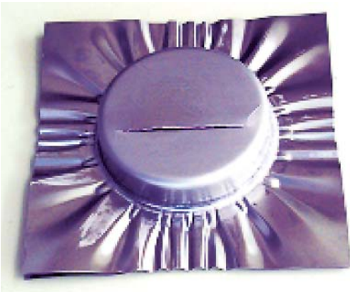
Figure 3: A pre-standard cup test specimen used at NIST to measure formability and constitutive behavior under equibiaxial strain conditions.
