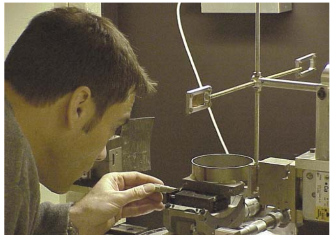
Figure 1: Residual stress measurement in Demeri cup at Advanced Photon Source.
