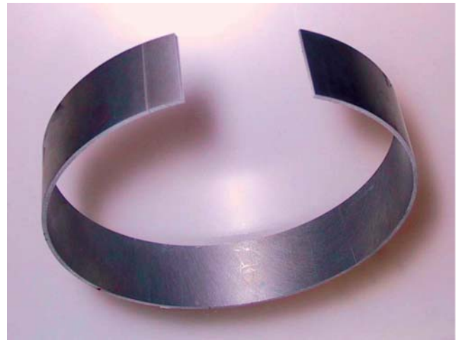
Figure 1: Split ring from Demeri cup springback test.
