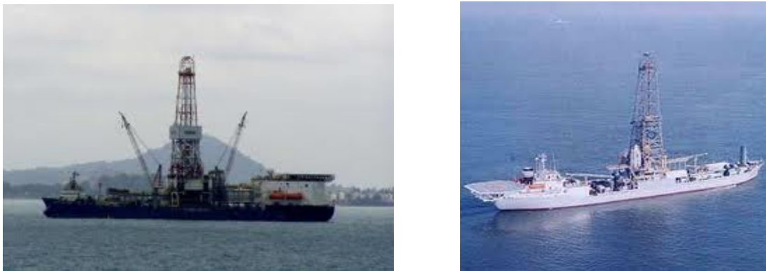
Figure 32: Conventionally moored Drillships
