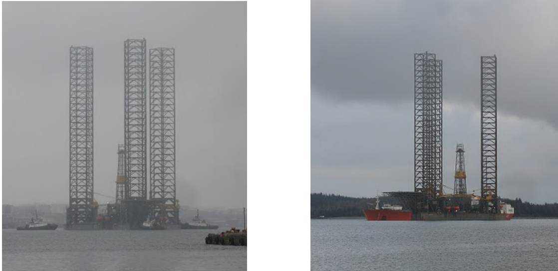
Figure 53: Tugs positioning the rig for float-on (left). HLV De-ballasting (right)
