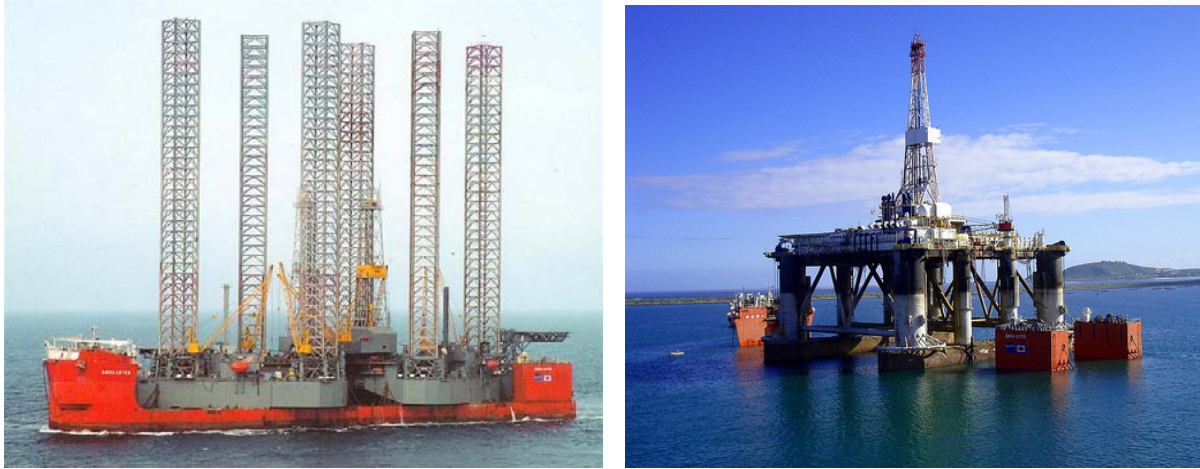
Figure 46: Barge Gavea Lifter (Two Jack-up Load to the left). Barge Gavea Lifter (Semi-Sub Drill Rig to the right)
