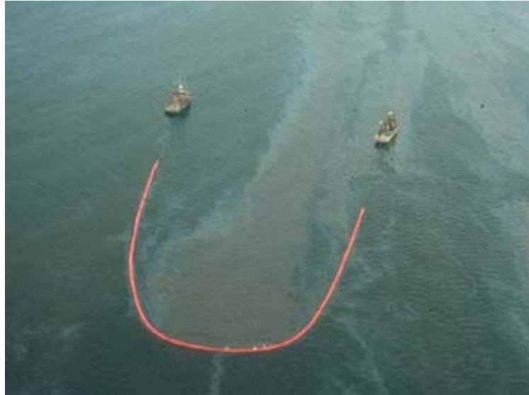
Figure 77: Containment techniques-U Shape Boom Configuration
