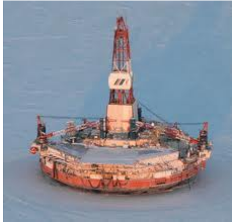
Figure 35: Ice-breaking drilling Barge-Kulluk
