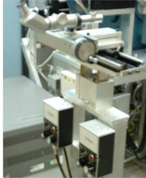
Chamber alignment controls mammography range
