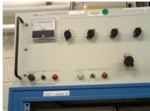
Wyckoff-Attix high voltage source
