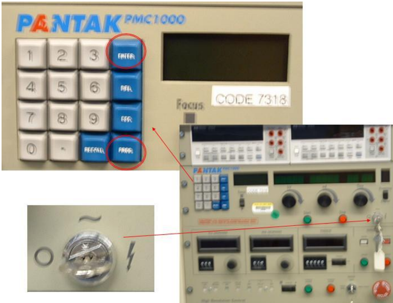
Figure 6. 100-300 kV x-ray controls.
