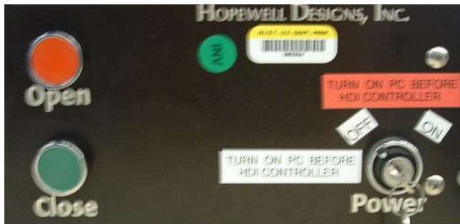
Figure 7. 100-300kV control panel and range control.
