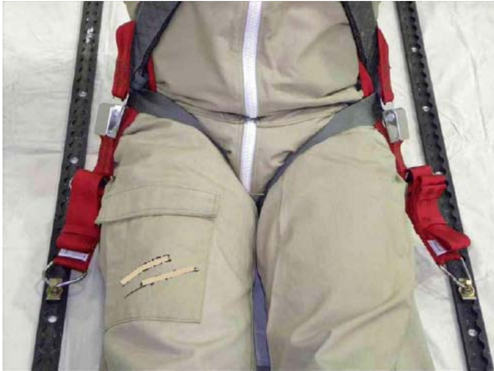
FIGURE 8. DUAL POINT, DUAL TETHER RESTRAINT ATTACHMENT TO FLOOR FOR REAR-FACING STRADDLE
