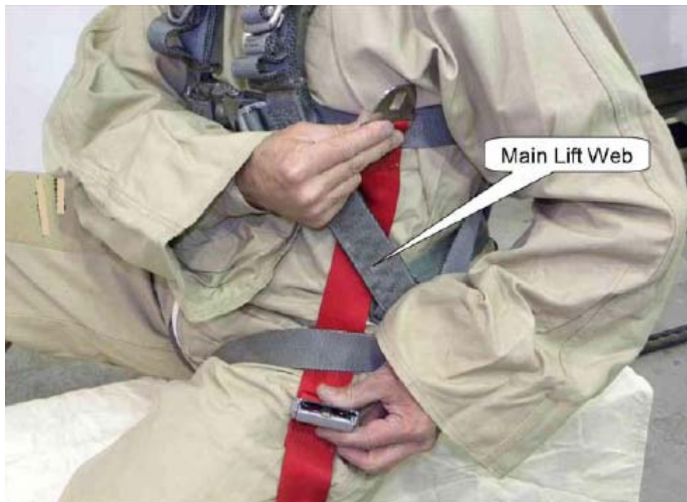
FIGURE 4. PASS TETHER LOOP UNDER MAIN LIFT WEB
