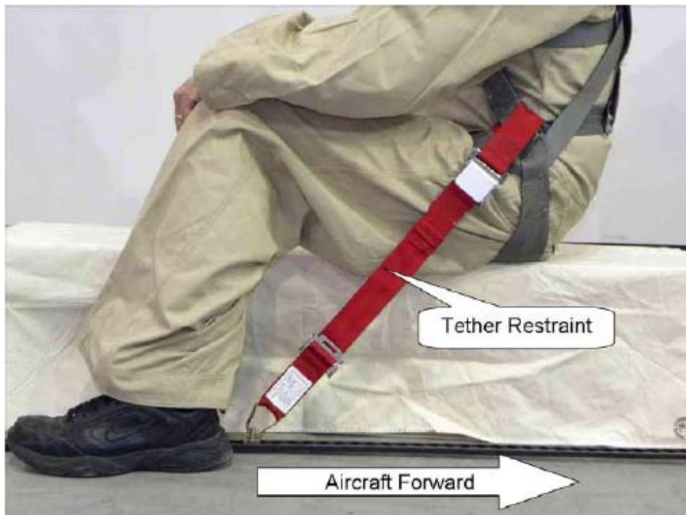
FIGURE 8. DUAL POINT, DUAL TETHER RESTRAINT ATTACHMENT TO FLOOR FOR REAR-FACING STRADDLE
