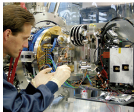
Figure 10. Timothy Jung works on the optical plate of the MDXR, which contains a cryogenic Fourier-transform spectrometer and other instrumentation necessary for absolute spectral calibrations.
