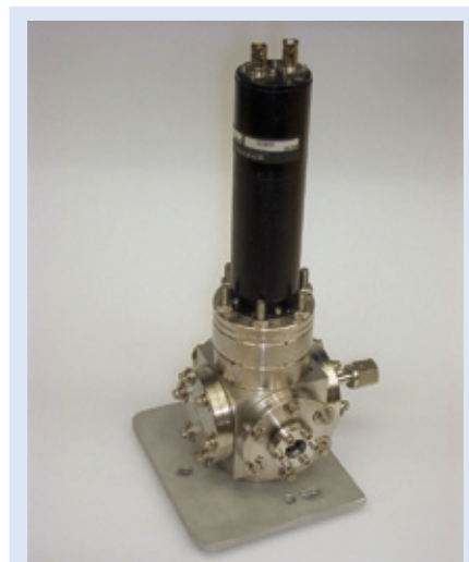
Figure 4. Lyman alpha radiation detector, shown here in prototype, could dramatically improve performance in key applications.
