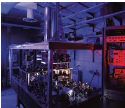
Figure 1. The NIST-F1 cesium-fountain primary frequency standard, the Nation’s standard for frequency and the SI second.
