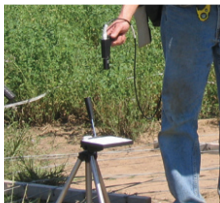
Figure 7. A researcher measures the solar radiance from a calibration plaque reflectance standard prior to measuring the reflectance of the terrain.
