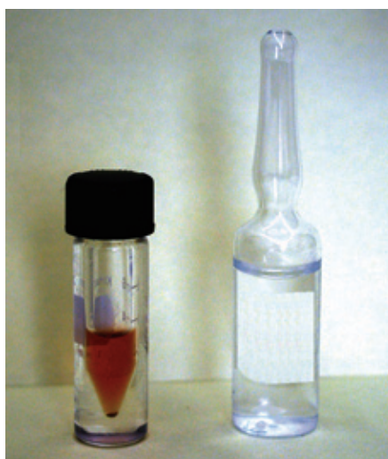
Figure 1. Sample vials of liquid radioactive sources used to study the calibration of portal monitors.
