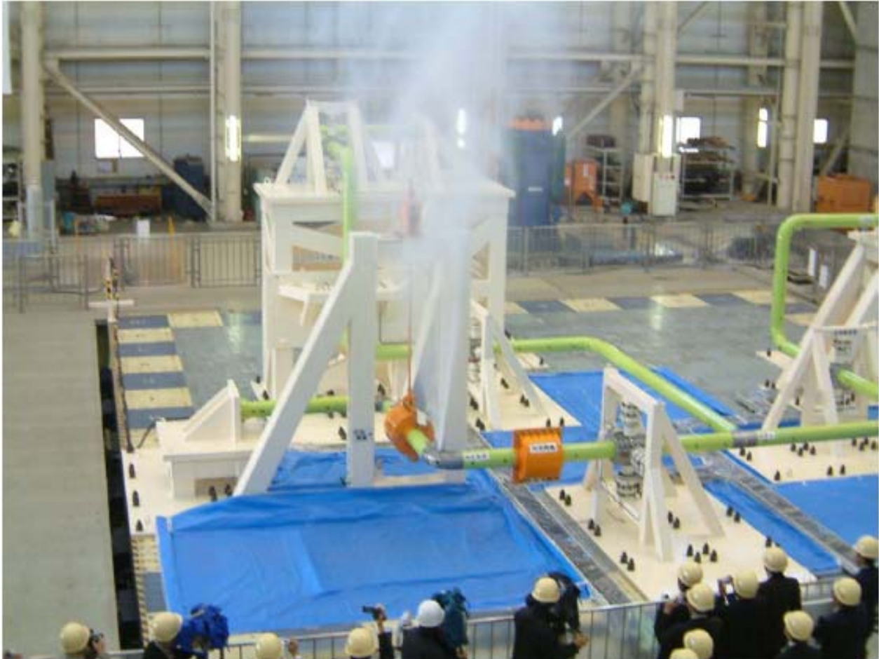
Figure 2-29 Ultimate Strength Test piping Failure at Elbow 2
