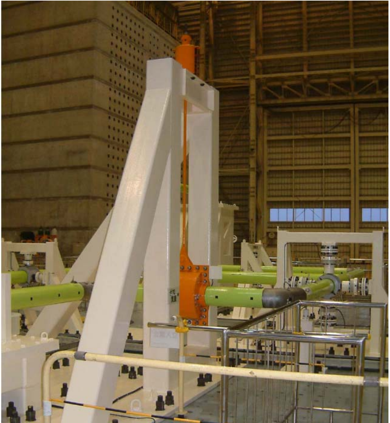
Figure 2-13 DM Test Spring Hanger
