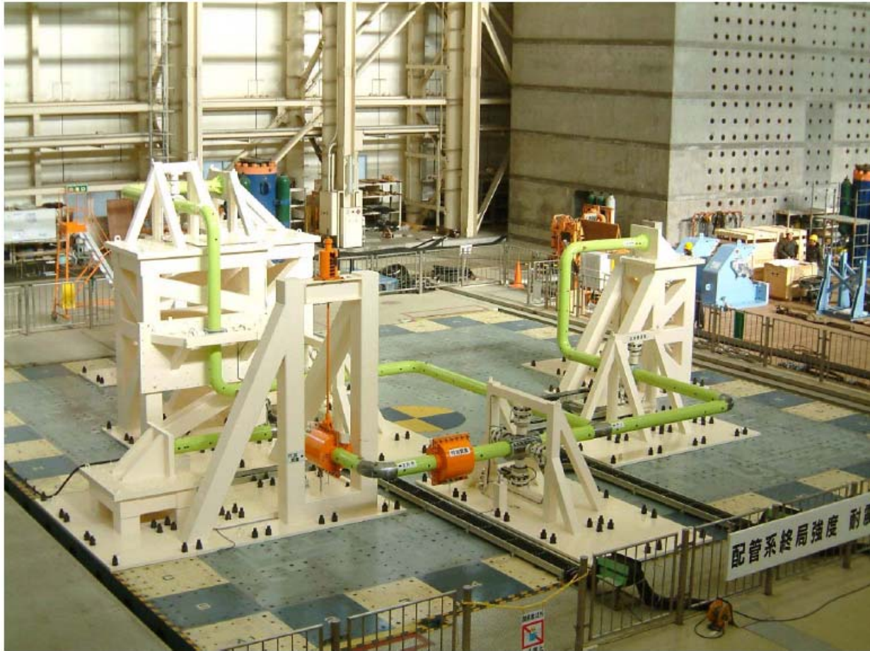
Figure 2-20 Overview of Ultimate Strength Test Piping System
