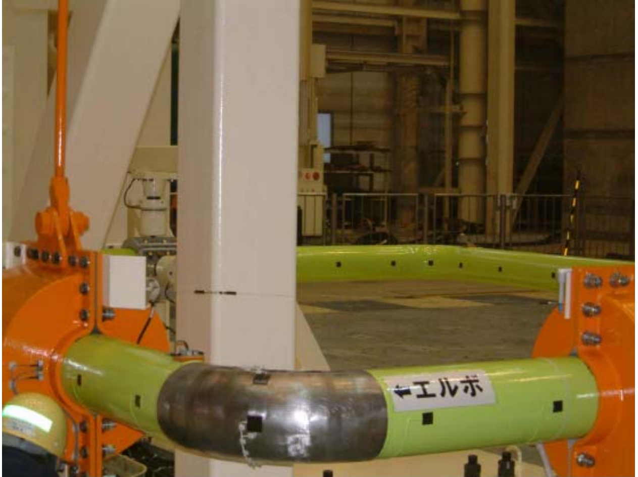
Figure 2-21 US Test Elbow 2 and Added Masses
