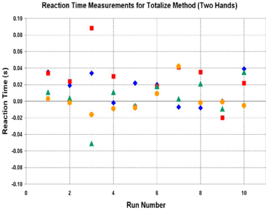
Figure 15. Measured reaction times (four operators, 10 runs each) for totalize method.
