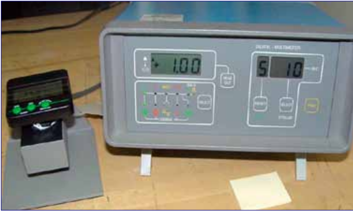
Figure 20. Time base measurement system for stopwatches and timers.
