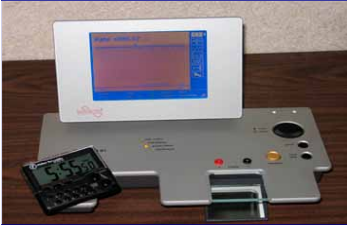
Figure 21. A time base measurement system for stopwatches and timers with an integrated graphics display.
