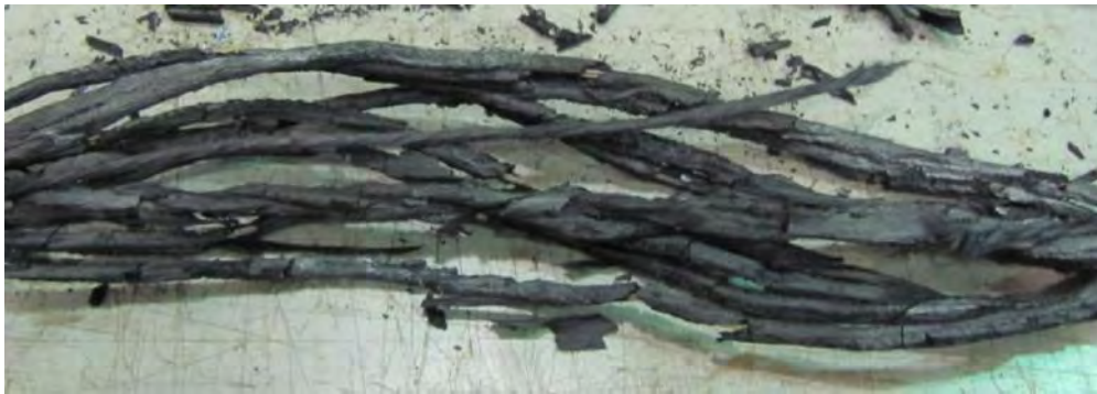
Figure 7.33: Conductors of Item G spread apart after Test K3.
