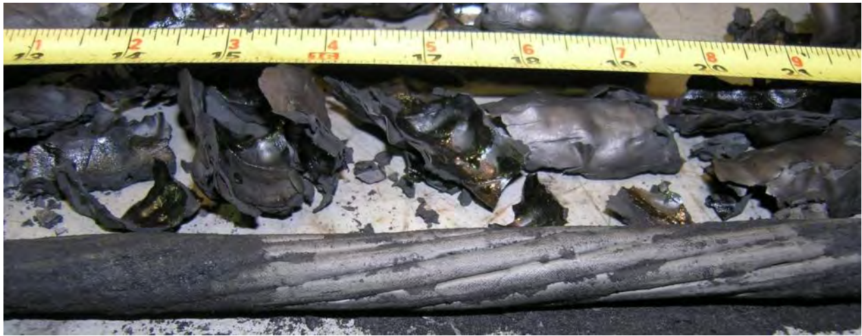
Figure 7.48: Post-test image of the conductors without insulation cracking for Item H.
