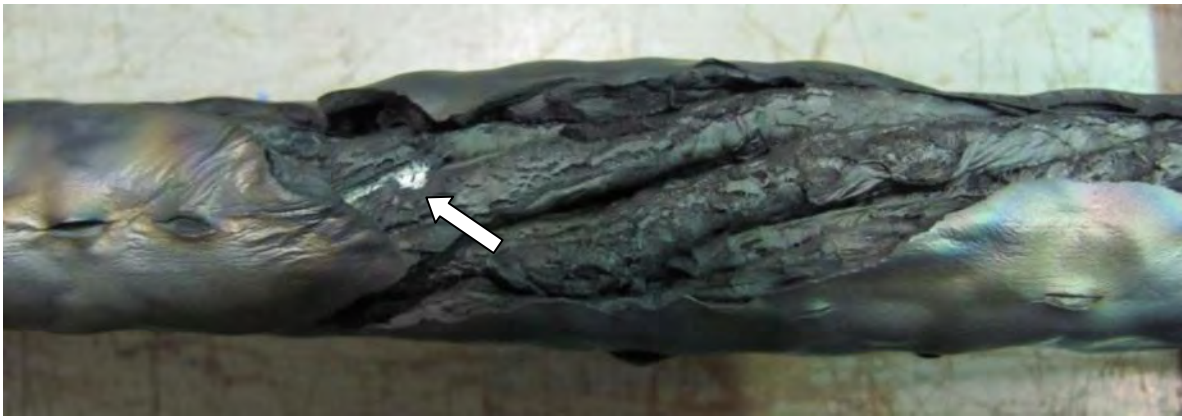
Figure 7.32: Close up view of the presumed failure point.
