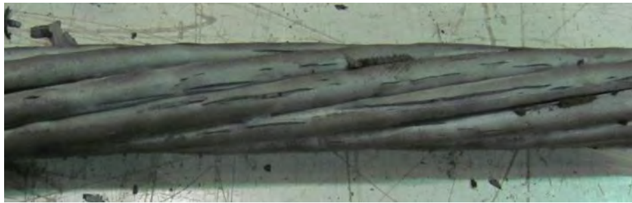
Figure 7.29: Longitudinal cracking observed during post-test analysis of Item F.
