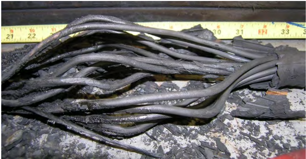
Figure 7.54: Opposite unburned section of Item I next to the leading flame edge.
