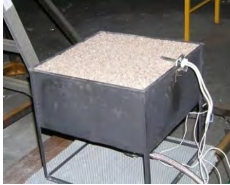
Figure 5.5: Photo of the sand diffusion burner.
