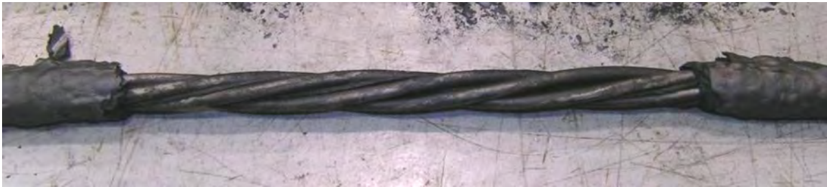
Figure 7.9: Post-test analysis of conductors from Item C located in the center of Penlight during Test K10 – no insulation cracking evident.
