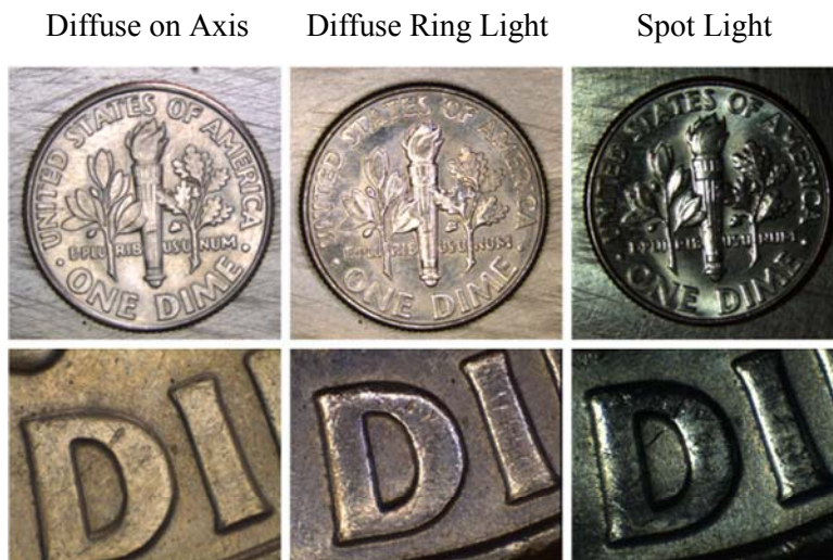
Figure 3.3 Dime Illuminated Using Three Lighting Techniques
