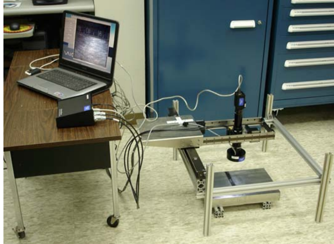
Figure 3.1 Visual Testing Apparatus and Sample
