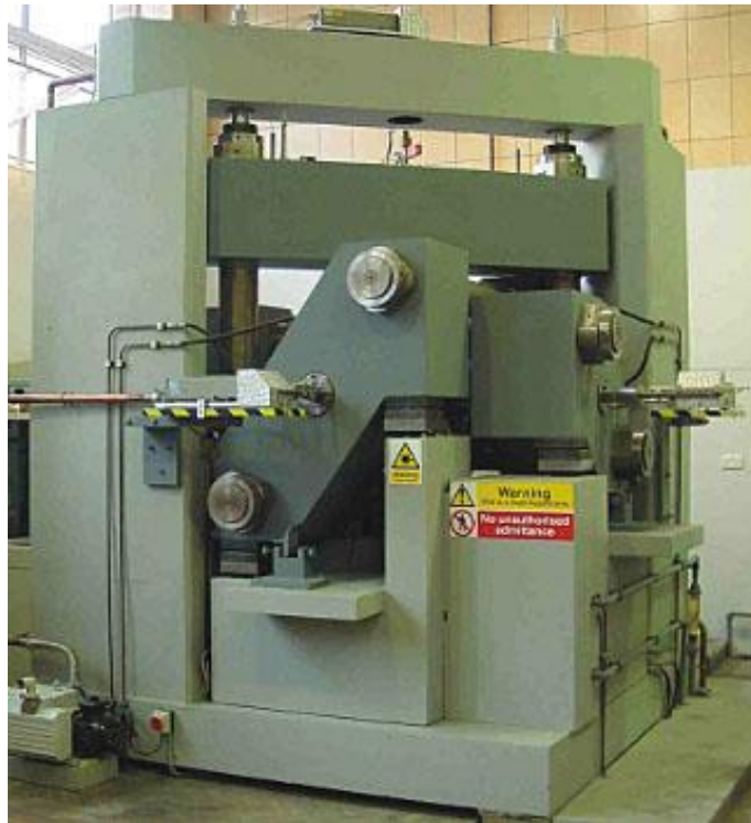
Figure 2.233 mac^{2T} apparatus for multiaxial compression of concrete at elevated temperature.
