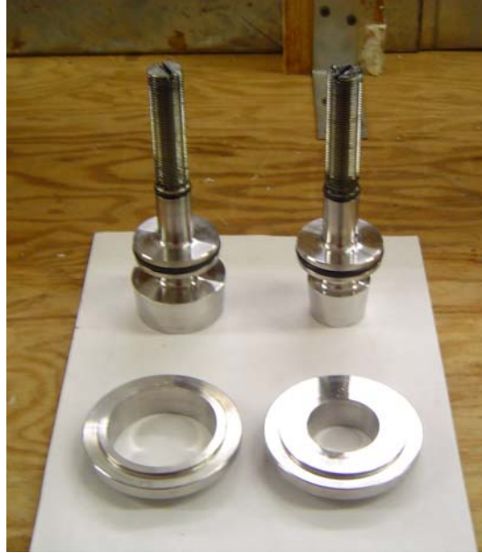
Figure 2-16. 5L and 5S Valve Stem-Seat Plugs and Seat Rings
