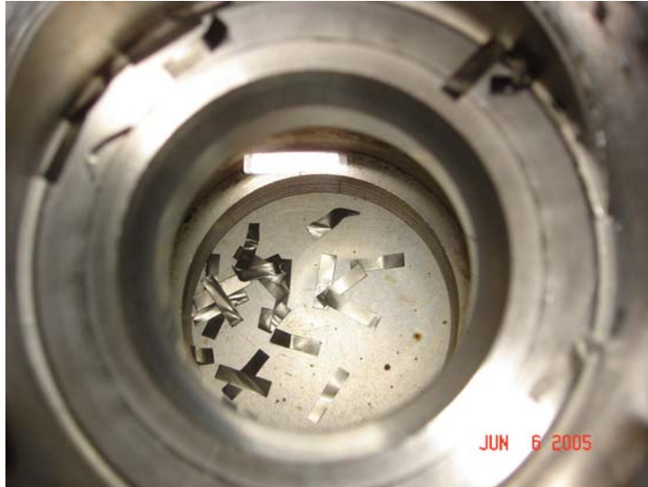
Figure A-2. Debris Found in the Valve Body Following an RMI Single-Debris Test
