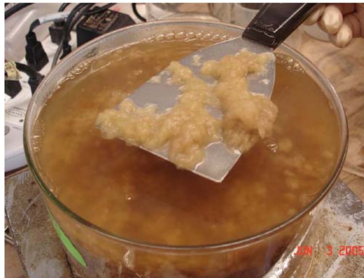
Figure 2-22. NUKON after Processing by Kitchen Blender
