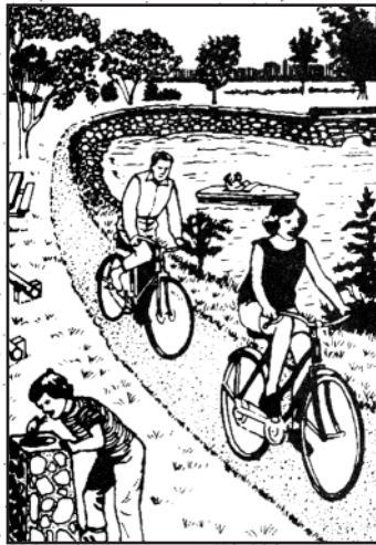
Gravel pit reclaimed as a lake and park; asphalt and crushed stone used for bicycle path along shoreline; stone used for a drinking fountain; stone (rip rap) used for protecting the shoreline from erosion.
