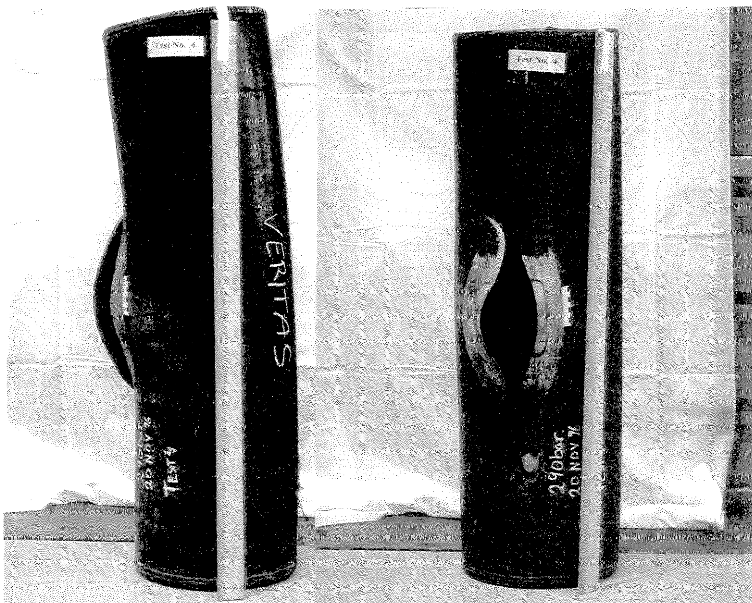
Figure 4-17 Picture of the test specimen no. 4 after the burst test
