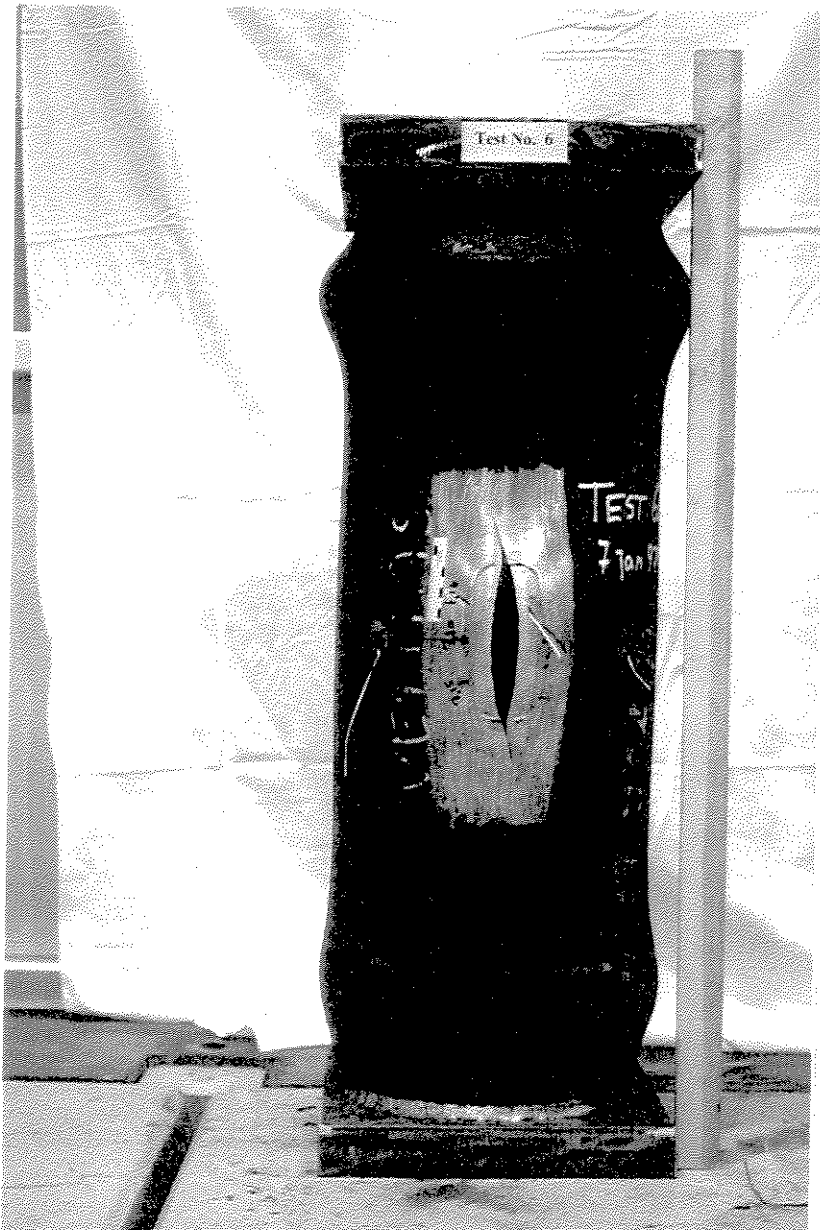
Figure 4-28 Picture of the test specimen no. 6 after the burst test
