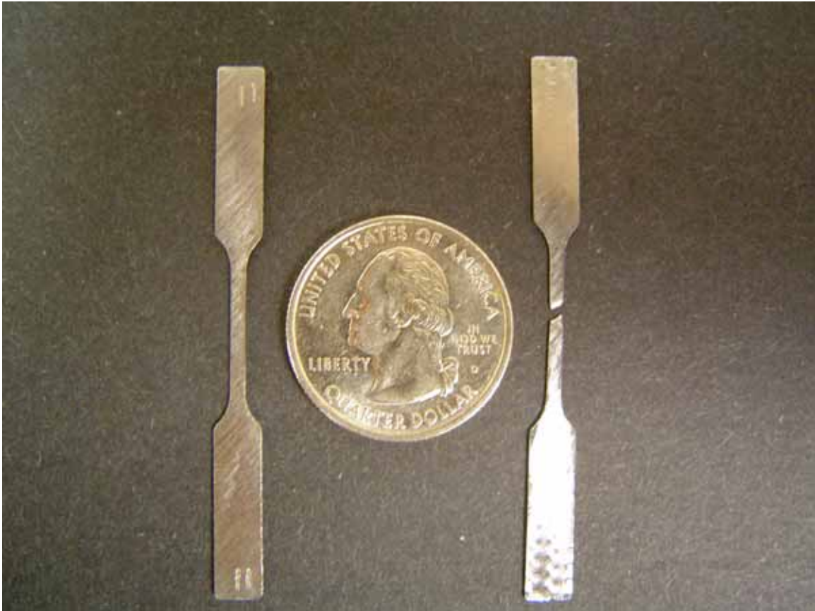
Figure 13. Examples of Microtensile Specimen Before and After Tensile Testing
