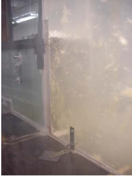
(i) Debris transport and accumulation on screen.
