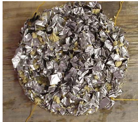
Figure 3.24. CalSil/RMI debris mixture in a typical 1-in. debris bed.
