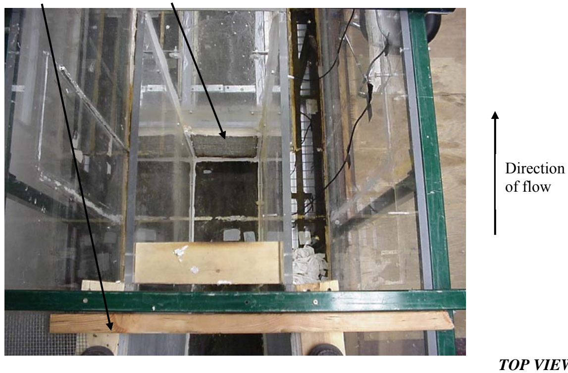
Figure A.3. Flume arrangement from end of converging section through the flow exit tunnel.
