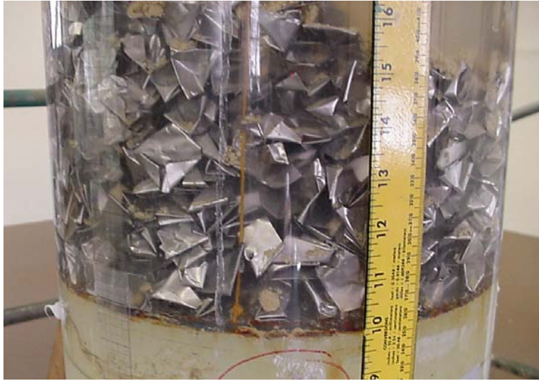
Figure 3.25. CalSil/RMI debris mixture in a typical 8-in. debris bed.
