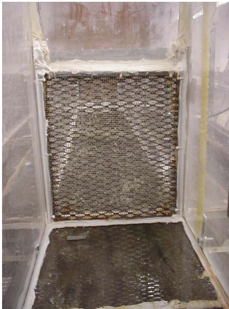
Figure A.2. Debris screen at entrance to flume exit tunnel (large, diamond-shaped mat behind screen is for structural reinforcement only).
