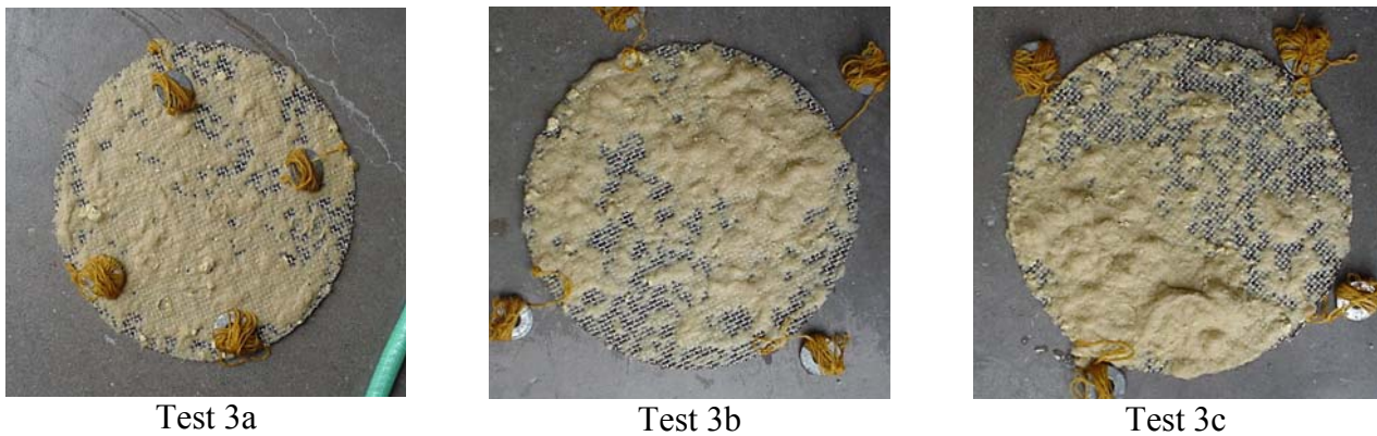
Figure 3.13. Post-test debris distribution on horizontal screens in thin-bed mixed debris Tests 3a-c.
