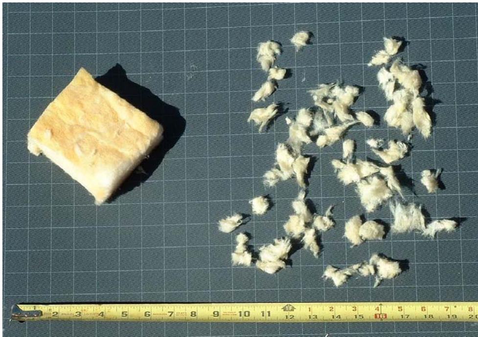
Figure C.1. NUKON™ fiber debris samples.
