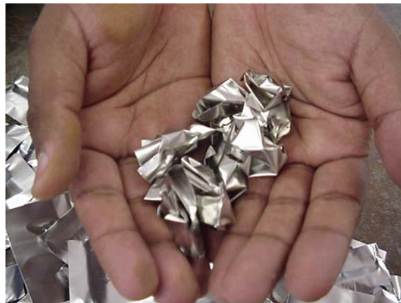
Figure C.5. Stainless-steel RMI debris used in experiments.
