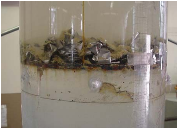
Figure 3.24. CalSil/RMI debris mixture in a typical 1-in. debris bed.
