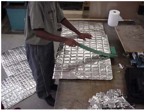
Figure C.3. Cutting RMI foil.
