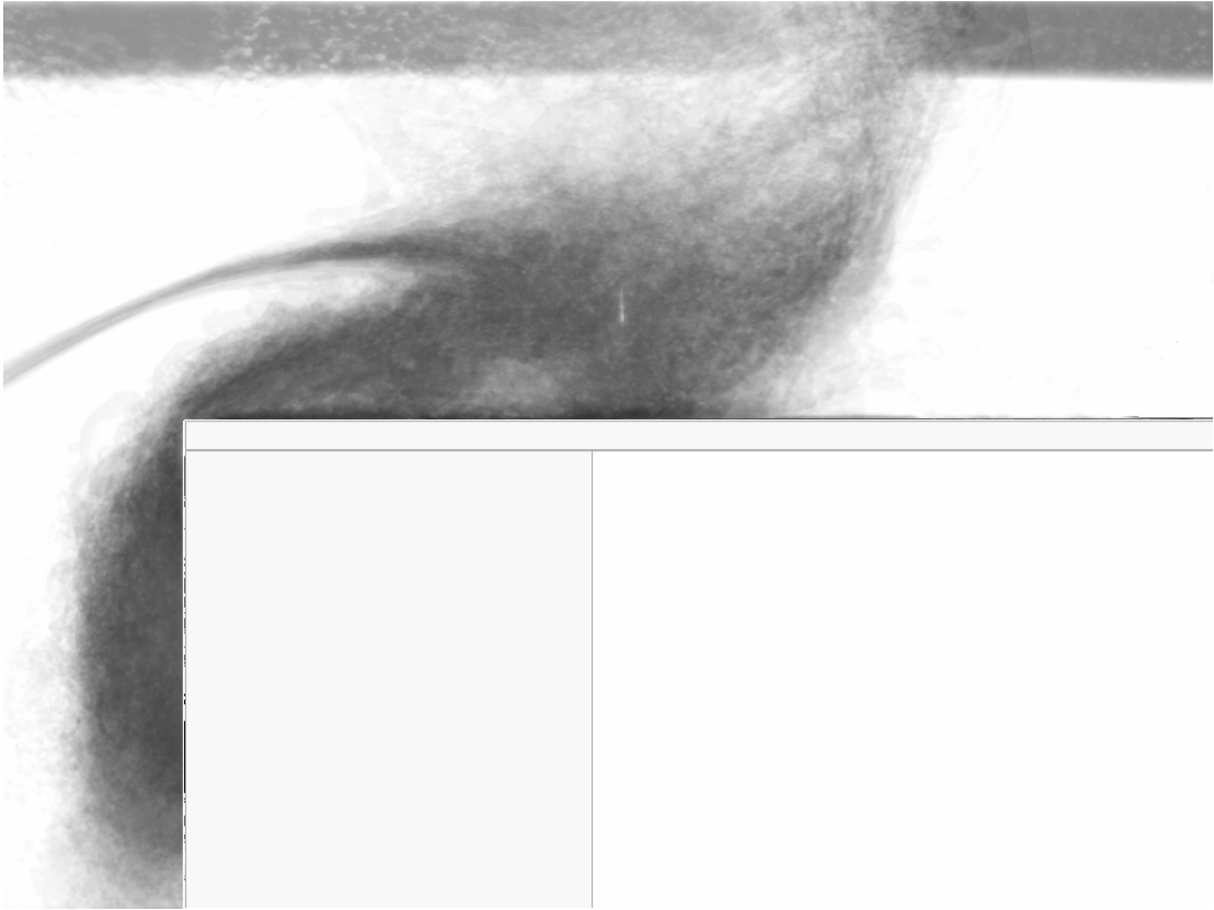
Figure 10.4 Sample ensemble averaged image of overtopping water on the deck.
