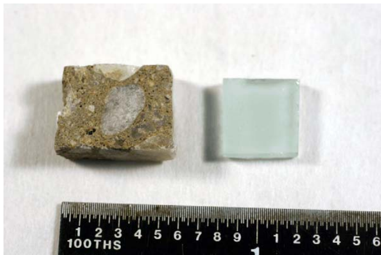
Figure B-2. Photograph Showing the Representative Nukon® Glass (Right) and Concrete (Left) Test Samples. Scale in Inches.
