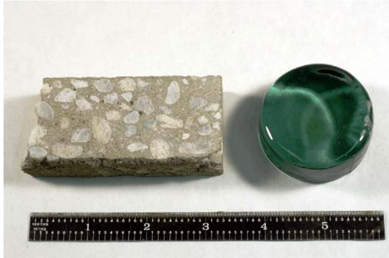
Figure B-1. Photograph Showing the As-Received Concrete Block (Left) and Nukon® Glass (Right) Samples. Scale in Inches.
