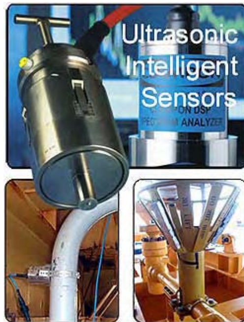
Figure 5.8: Subsea sand monitors 17 .
