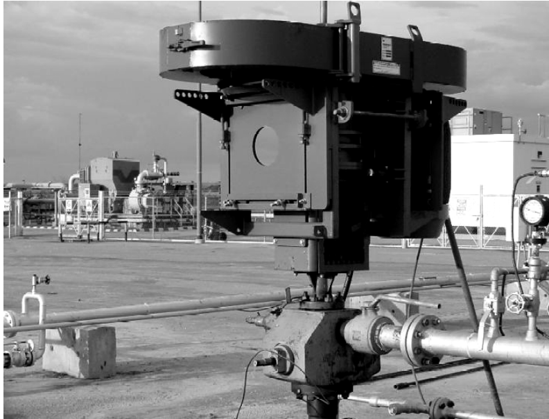
Figure 9.7: This field in a Petrozuata oilfield (Venezuela) combines conventional downhole pumping with surface multiphase pumping.
