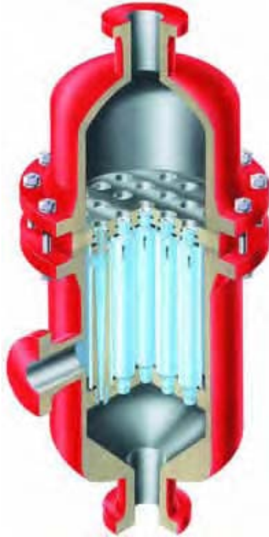
Figure 4.6: Cutout of a desanding multi-cyclone 49 .
