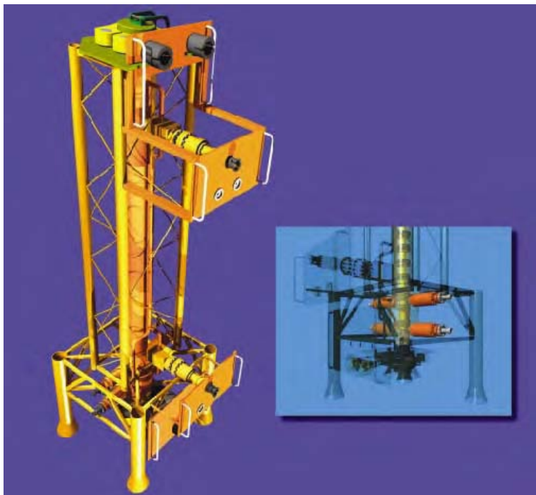
Figure 5.6: Equipment for single trip pigging 56 .
