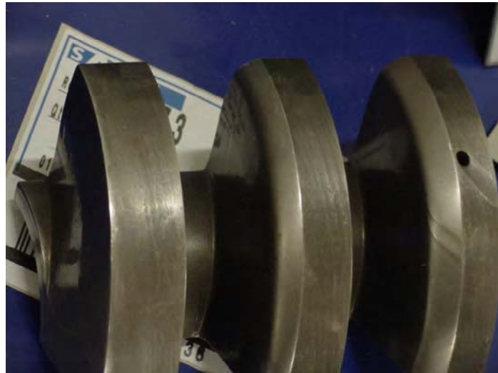
Figure 3.31 – Wear Caused by Sand Production
