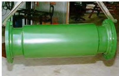
Figure 5.10: North Sea MFC designed for 10000 BOPD 56 .
