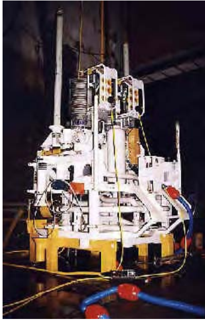
Figure 2.12: A subsea multiphase pump module 10 .
