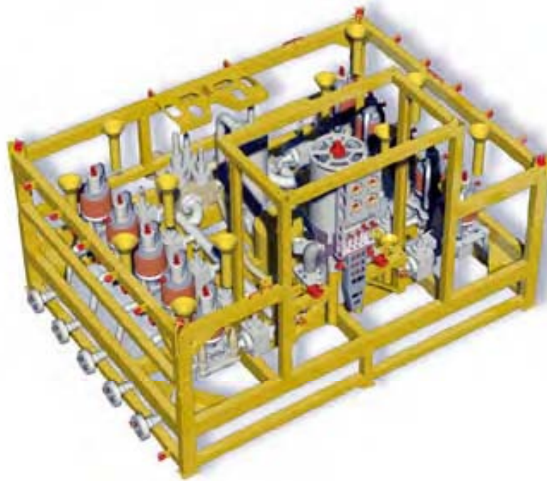
Figure 3.13: Mutineer Subsea Multiphase Pump/Meter Module
