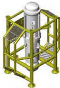
Figure 2.11: Schematic of a subsea gas compressor 5 .
