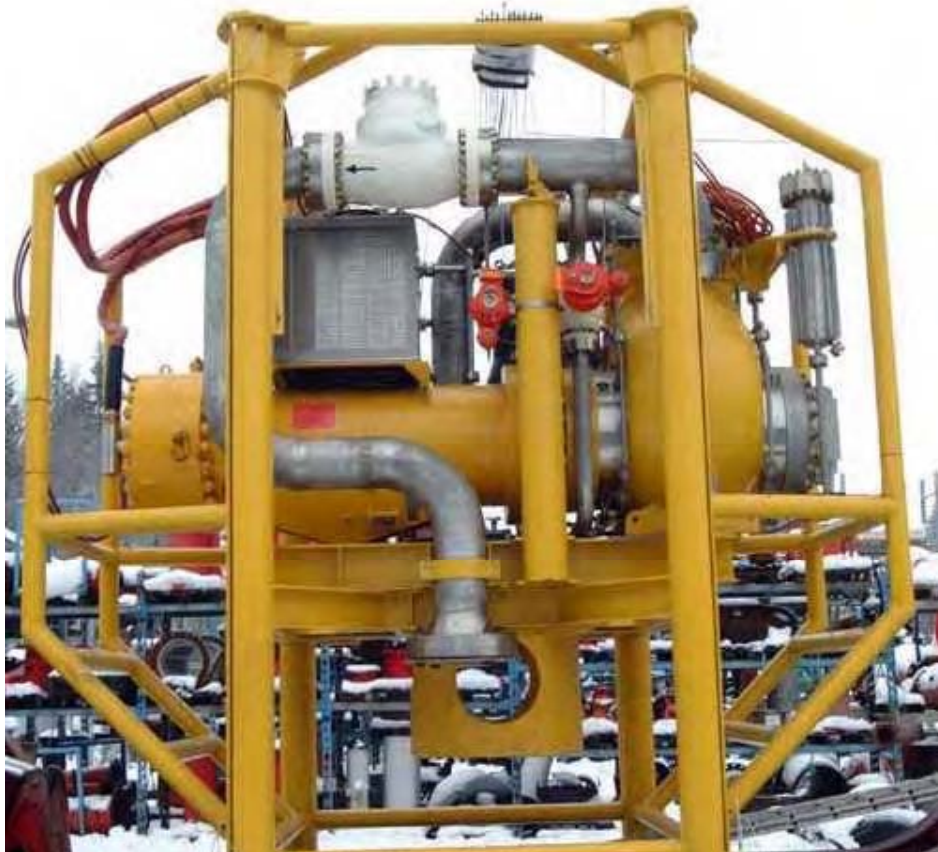
Figure 3.18: AkerKvaerner Subsea Pump Module with Bornemann Pump
