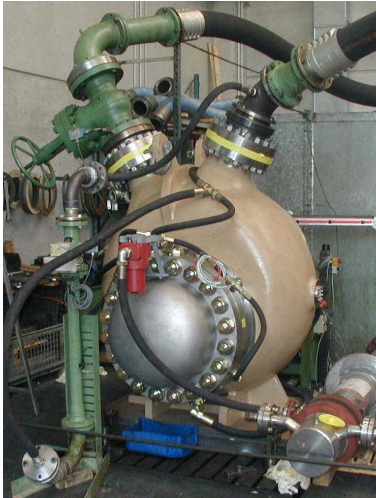
Figure 3.19: Bornemann Subsea Multiphase Pump on Test Stand
