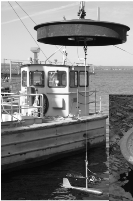
800 lb weight with current meter goes on first. Tow boat in background.
