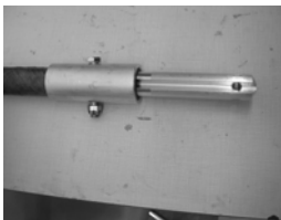
Pipe end with rod and bolt & Groove for cable
