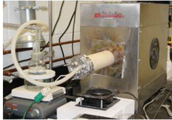
Figure 4. Tube furnace used for exposure testing of samples in a flowing stream of hot, moist air.
